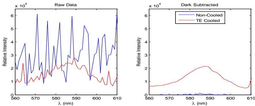
**Figure 2:** A comparison between a non-cooled (blue) and TE-cooled (red) spectrometer showing the fluorescence spectra of a quantum dot made up of a cadmium selenide (CdSe) core and a zinc sulfide (ZnS) shell, engineered to fluoresce at 584nm. The plot on the left shows the raw data (noise included), while the plot on the right shows the spectra with the dark noise subtracted out.
