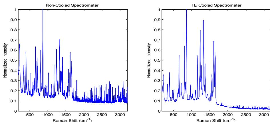
**Figure 3:** Raman spectrum of acetaminophen collected using a non-cooled spectrometer (left) and a TE-cooled system (right)
