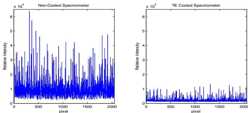
**Figure 1:** Dark current noise for a non-cooled CCD spectrometer at room temperature (left) and a TE-cooled CCD spectrometer at 14°C (right), using an integration time of 30 seconds
