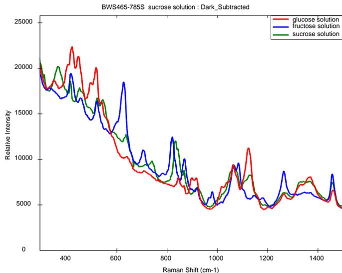
**Figure 1:** Raman spectra of aqueous sugar solutions
