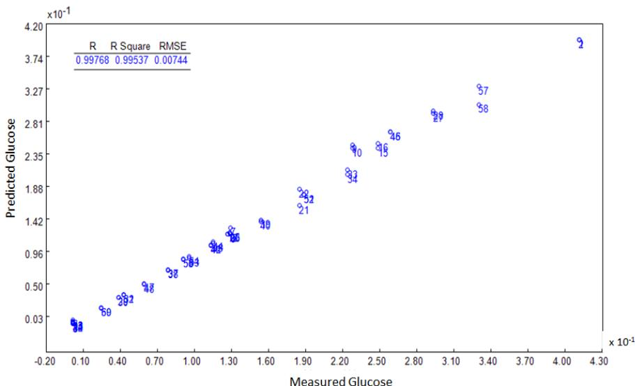
Figure 3: Measured vs. predicted plot of concentration percentage for Glucose 3 Factor PLS model
