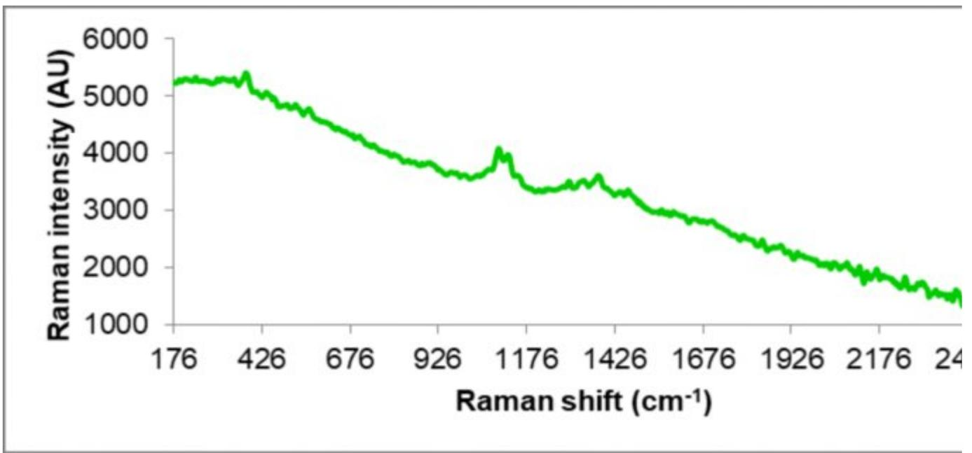
Figure 1. Raman spectrum of a suspected counterfeit Adderall pill collected with a 785 nm handheld Raman system
