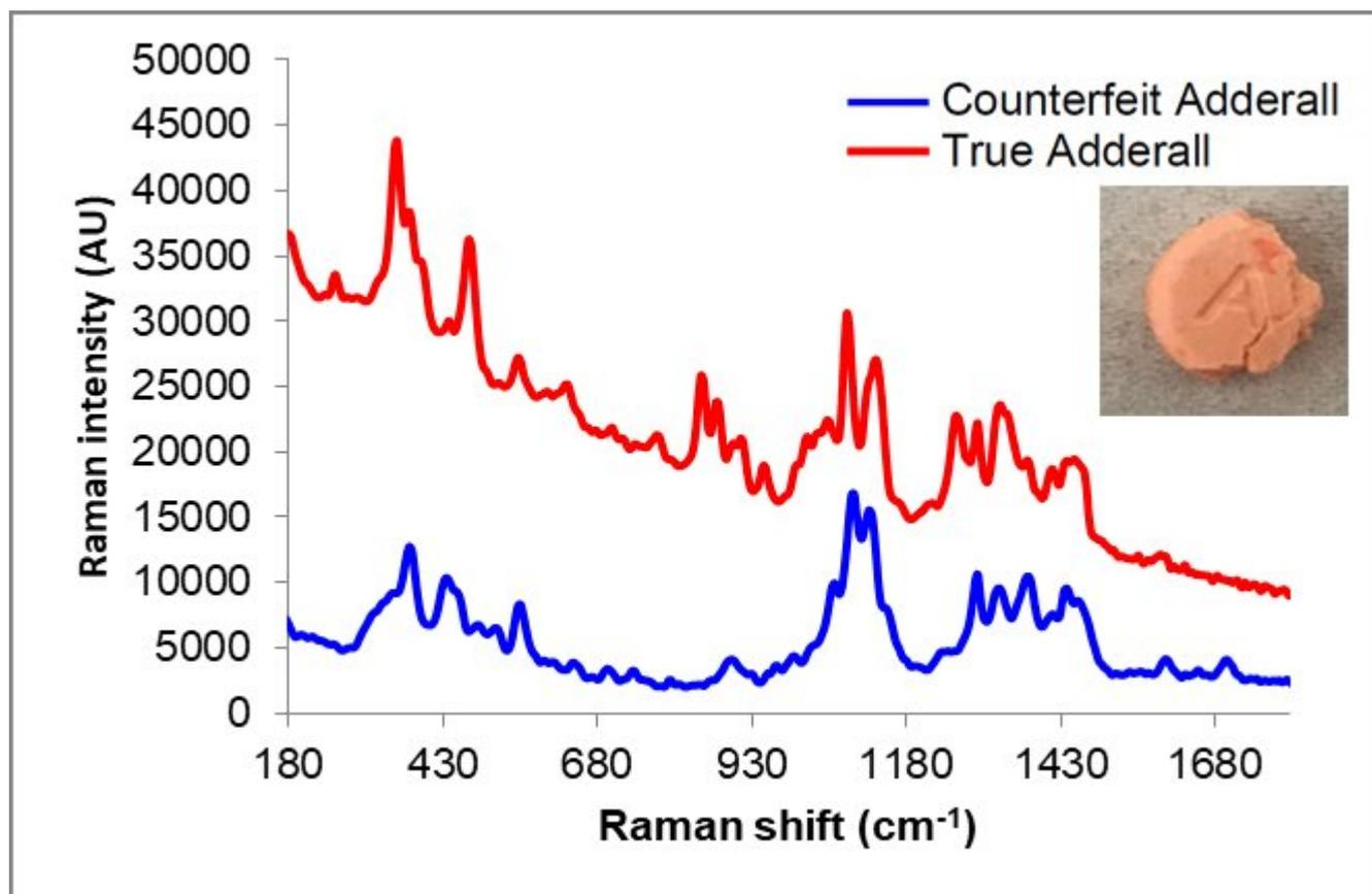
**Figure 3.** TacticID Mobile spectra of suspected counterfeit Adderall compared with a true Adderall pill (Insert: photo of suspected counterfeit pill. The color and markings match true Adderall pills.)
