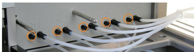
**Figure 94.** The connections on the back wall for the five solvent tubes connected to the solvent feeder.
