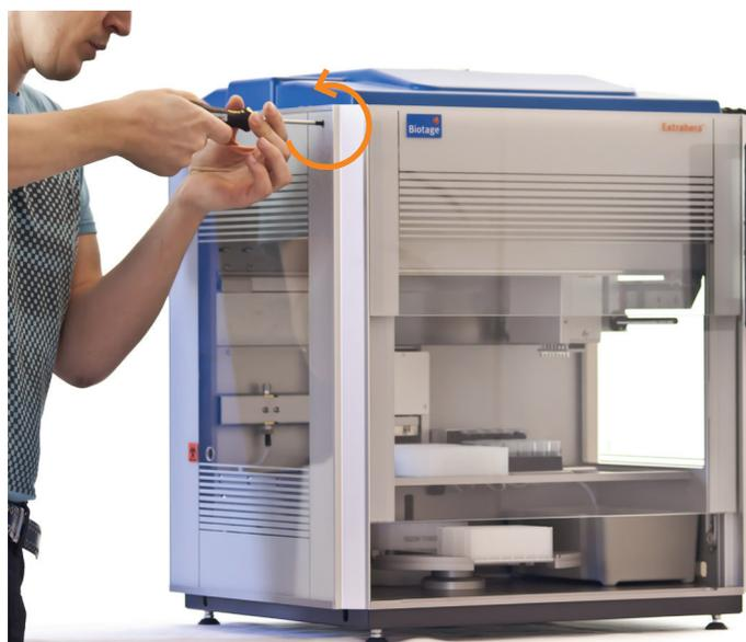
**Figure 7.** Open the door manually by turning the screw counterclockwise using the T25 Torx screwdriver supplied with the system.
