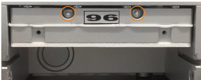
Figure 100. The two screws attaching the pressure head to the pressure unit.
