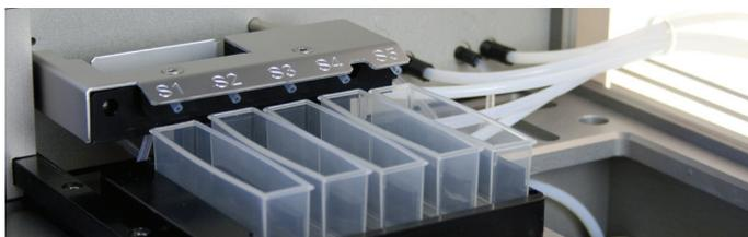
Figure 96. The solvent feeder in position.
