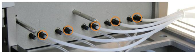
**Figure 93.** The solvent inlet connections at the back wall.
