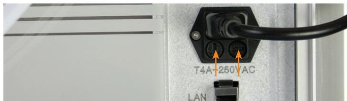
Figure 102. Fuse holders at the power inlet.
