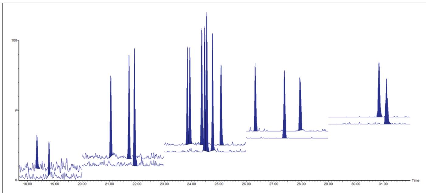
Figure 1. Example of chromatographic separation achieved for 17 PCDD/DF congeners at 1 in 10 dilution of the CSL standard.
