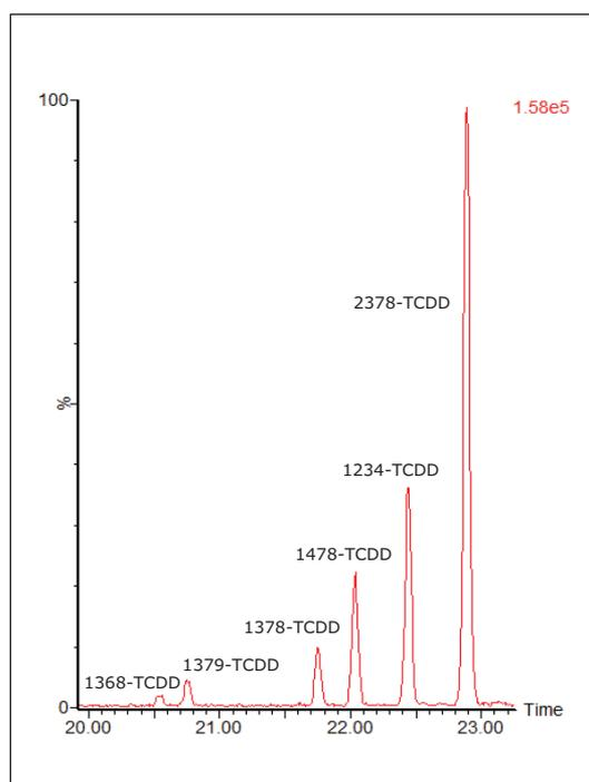
Figure 2. Chromatographic separation of TCDD congener mix containing 2 to 100 pg (concentration on column, with 1  $\mu\text{l}$  injected).
