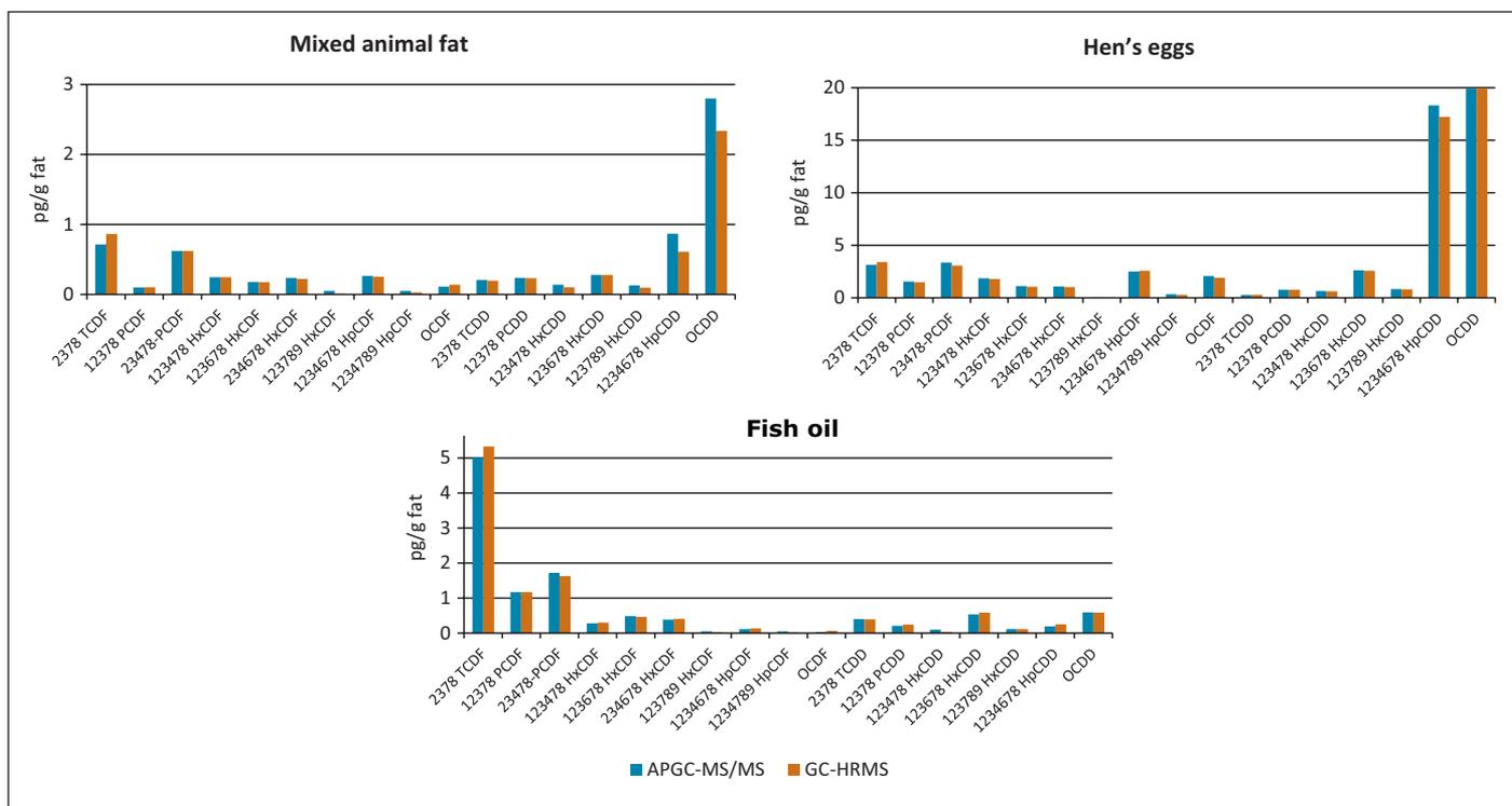
Figure 4. Comparison of results obtained from APGC-MS/MS and GC-HRMS for a sample matrix of mixed animal fat, fish oil, and hen's eggs.
