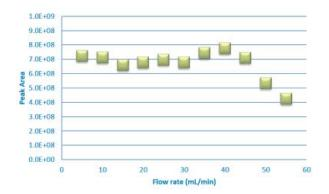
Figure 9. Flow rate optimization for sampling of  $10\mu L$  formaldehyde/ $H_2O$  solution out of a 10 mL vial.
