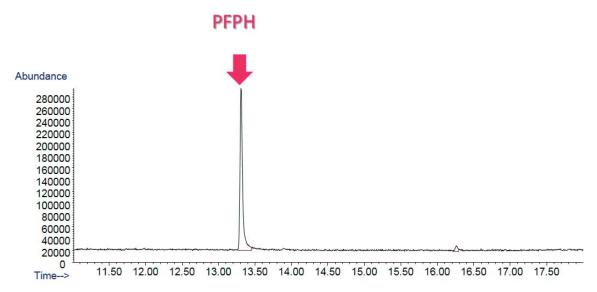
Figure 5. Chromatogram resulting from injection of 1 µL PFPH stock solution directly into the CIS/PTV inlet.
