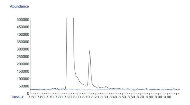
Figure 7. Comparison of a chromatogram obtained from thermal desorption of a Tenax TA tube loaded with 100 µL PFPH and a background chromatogram of the same Tenax TA tube desorbed directly afterwards (blue chromatogram).
