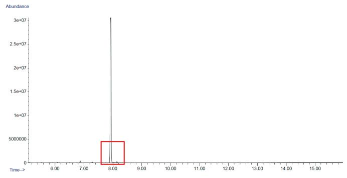
Figure 6. Peaks of PFPH and PFPH-formaldehyde after DHS loading of 100 μL PFPH stock solution and split 1/40.
