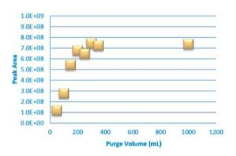
Figure 10. Purge volume optimization for  $10\mu L$  formaldehyde/ $H_2O$  solution in a 10 mL vial.
