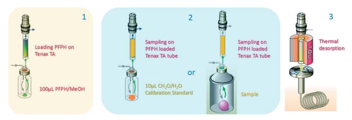
Figure 2. Schematic drawing of the PFPH/TD-GC/MS method steps.
