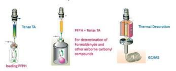
Figure 13. PFPH/TD-GC/MS: Schematic diagram of the method used for determination of formaldehyde and other airborne carbonyl compounds.
