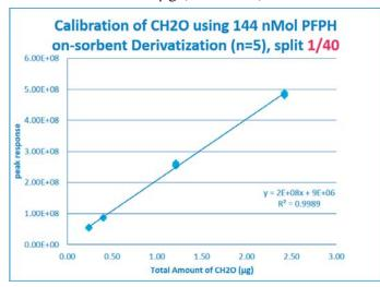
Figure 11. Formaldehyde calibration curve linearity (4 levels, n=5 each).
