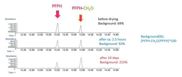
Figure 4. Chromatograms obtained after different drying periods for PFPH-loaded tubes placed in a fume hood.
