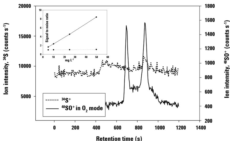
Figure 1. Upper left: S/N vs concentration for S with O<sub>2</sub> addition to the ORS. The method enabled identification of chromatographic peaks (<sup>48</sup>SO<sup>+</sup> signal) not seen in standard mode (<sup>34</sup>S signal).
