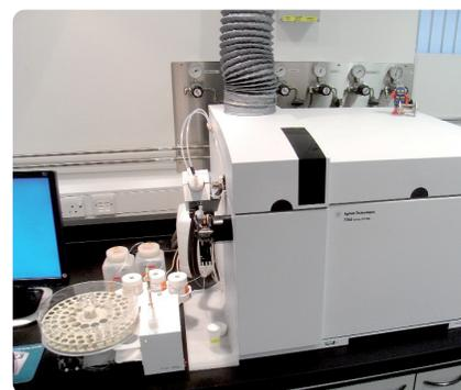
Figure 1. Agilent 7700x ICP-MS – capable of routine pharma applications, as well as more advanced studies for R&D facilities.
