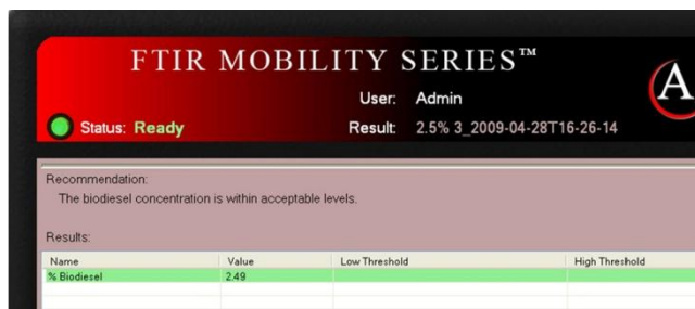
Figure 5. Microlab results screen for a 2.50 vol % sample of biodiesel in diesel
