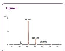
For pesticide analysis, the 6550 iFunnel Q-TOF demonstrated (Figure A) 10-fold sensitivity gain for a poor responding pesticide (fluazifop-butyl) in pepper matrix. Extracted ion chromatogram shows excellent detection (S/N 1200) on 10 ppb fluazifop-butyl and (Figure B) confident compound identification of fluazifop-butyl with an excellent library match score of 98 based on a mass error of only 0.5 ppm and correct fit of isotope abundance and spacing.
