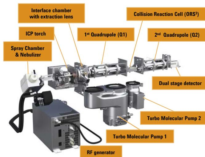
Figure 1. Configuration of Agilent ICP-QQQ
