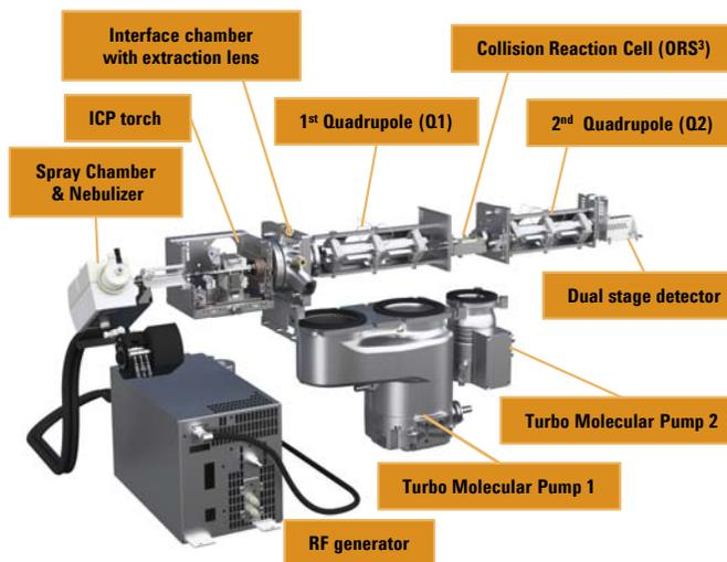
**Figure 1.** Configuration of Agilent ICP-QQQ
