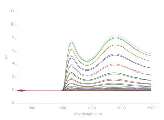
**Independent control of sample rotation and detector position** Diffusely scattered transmission through an AR coated silicon wafer with a polished front surface and unpolished back surface. Each spectrum is measured at a different angle either side of direct transmission, demonstrating the ability of the Cary 7000 UMS to move the detector around the sample.
