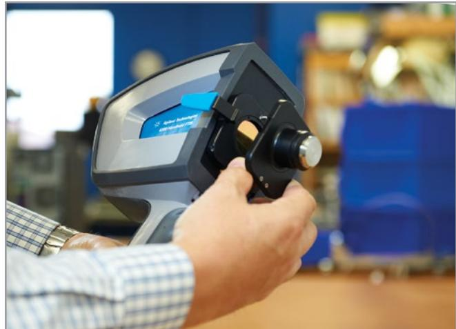
**Longer periods of continuous operation:** The lithium ion batteries that power the 4300 can easily be swapped while the system is running.
