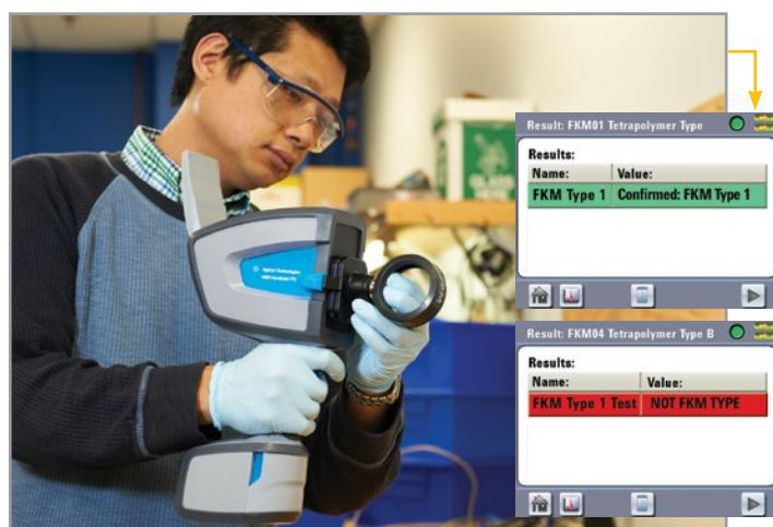
In the MicroLab method chosen for the pictured O-ring analysis, a threshold was set such that samples within the target group are shown in green while those outside the target group are shown in red. Furthermore, the conditional reporting feature can be used to display a customized alert message such as, "Confirmed FKM Type 1" for samples within the target group and the message "NOT FKM TYPE 1" for samples outside the target group.
