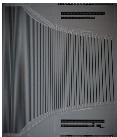
Figure 2. Custom-designed and proprietary CCD detector. With unique I-MAP and AIT, speed and versatility is unmatched, and full wavelength coverage is provided from 167–785 nm.
