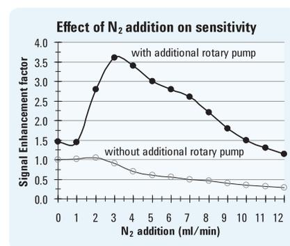
Figure 1. Effect of N<sub>2</sub> addition on sensitivity of <sup>238</sup>U.
