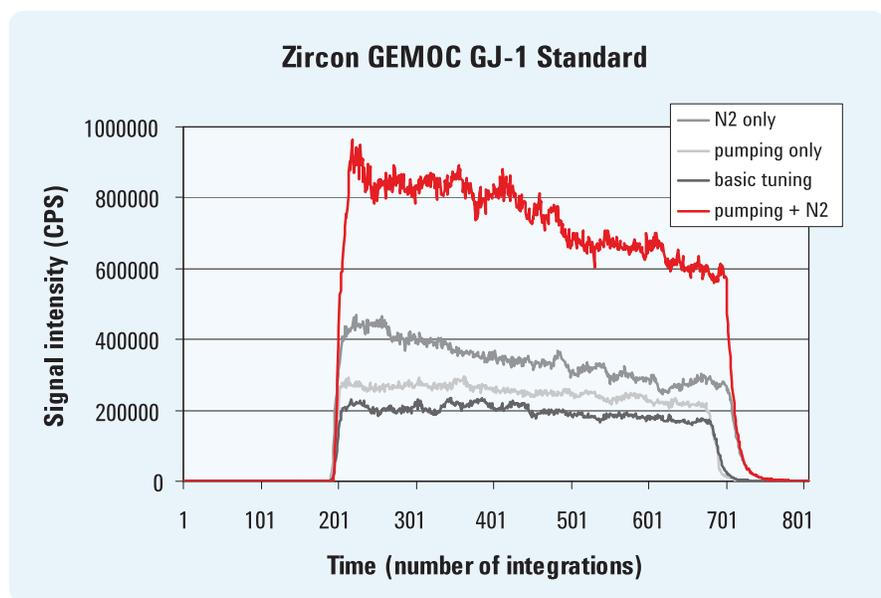
**Figure 2.** Time resolved profiles of  $^{238}\text{U}$  in zircon reference material GEMOC GJ-1.
