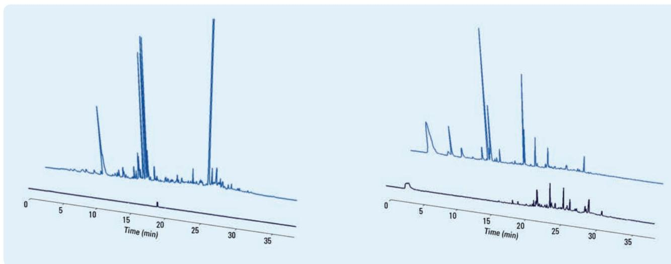
**Figure 2.**  $^{81}\text{Br}$  (Left) and  $^{127}\text{I}$  (Right) GC-ICP-MS chromatograms obtained from MTBE extracts prepared from a representative wastewater sample before chloramination (purple line, front) and after chloramination (blue line, behind). Intensity scales are identical for both plots. Chromatograms are not background-subtracted.
