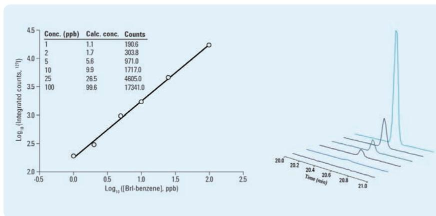
**Figure 1.** Log/log plot of a calibration curve for <sup>127</sup>I prepared from 1-bromo-4-iodobenzene (left panel) and an overlay of <sup>127</sup>I peak intensities for calibration standards (ranging from 0.0 to 25 ppb) examined in this work, including a calibration blank (right panel). The retention time for this compound is 20.6 minutes.
