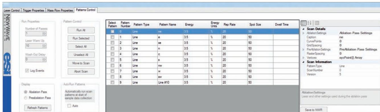
**Figure 2.** Detailed view of Pattern Control pane of the new ESI NWR ActiveView plug-in for Agilent ICP-MS MassHunter
