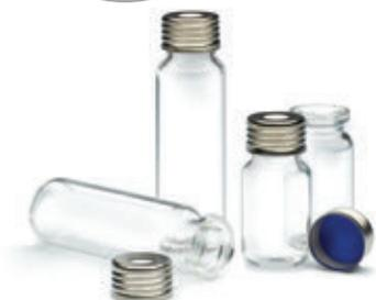
Beveled-neck headspace vials are available in both 10 mL and 20 mL capacities, flat or rounded bottom. The 20 mm crimp caps provide a consistently secure seal. Agilent also offers cost-saving convenience packs with vials, caps, and septa packaged together.
