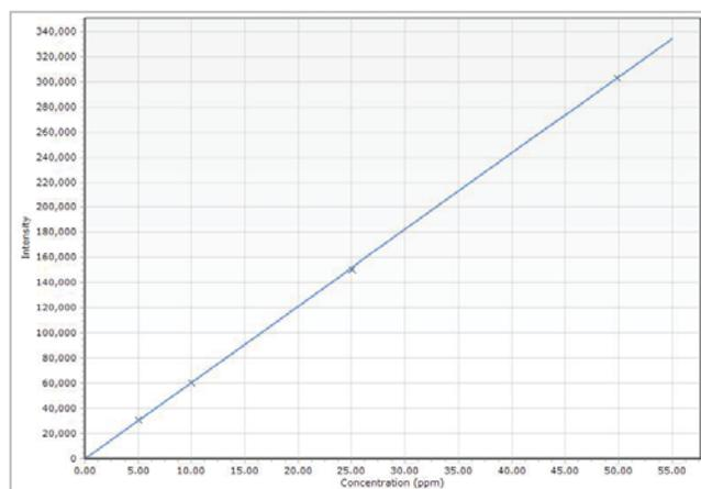
**Figure 1.** The calibration curve for Ca 422.673 nm up to 50 ppm shows excellent linearity across the calibrated range, with a correlation coefficient of 0.99998.
