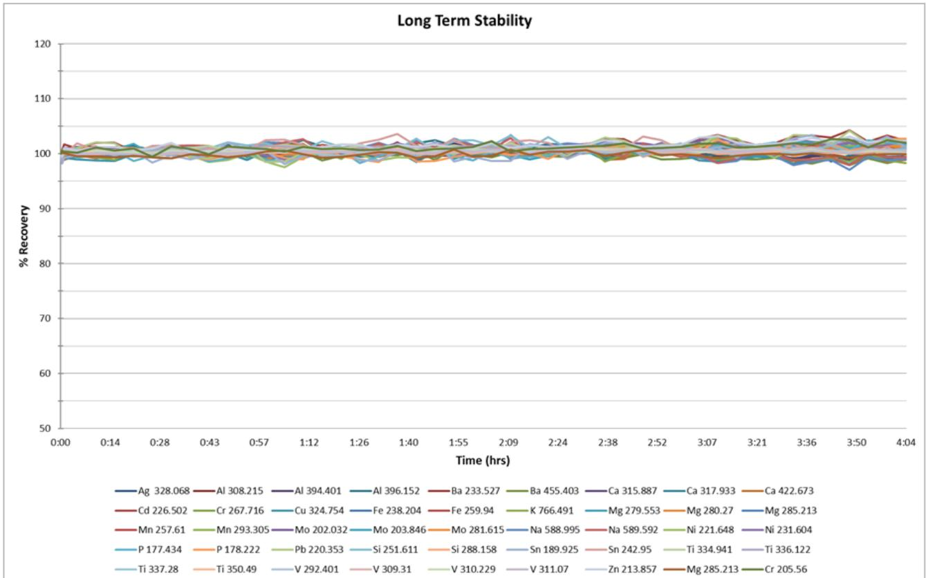
**Figure 2.** Stability plot over 4 hours for all elements in a used oil sample using the 5100 RV ICP-OES
