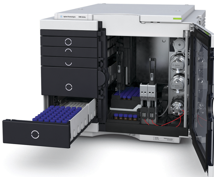
Figure 1. Design and interior of the Agilent 1290 Infinity II Multisampler.
