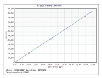
Figure 3. Calibration curve for Ca (422.673 nm) in oil diluted in kerosene.
