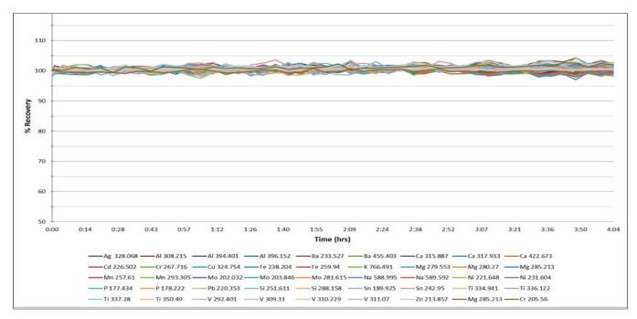
Figure 1. Long-term stability plot for all wavelengths of a 5 ppm multi-element organometallic standard in kerosene.
