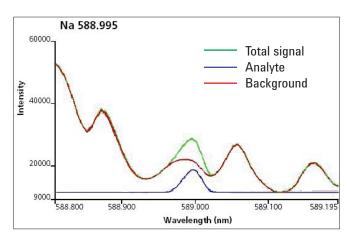
Figure 4. FACT background correction on Na (588.995 nm) in a used oil sample.
