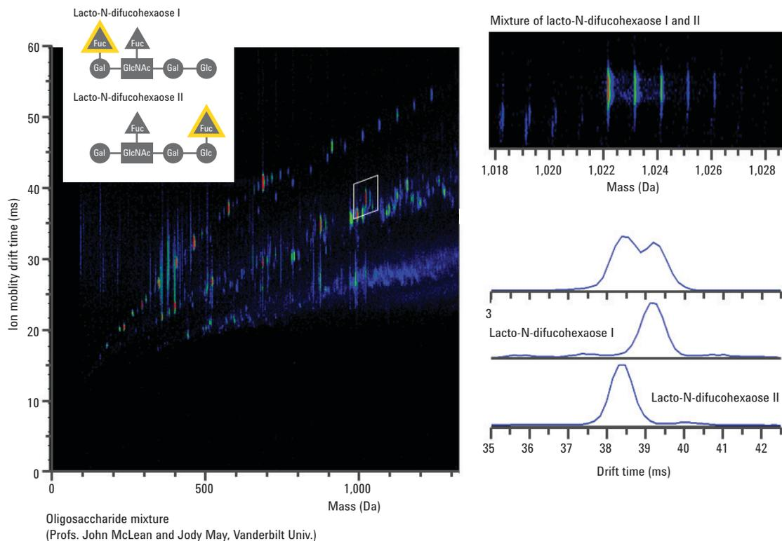
A mixture of lacto-N-difucohexaose I/II isomers, which differ by the location of the fucose group, is discovered in a complex sample mixture using the 6560 IM-Q-TOF. Upon individually analyzing the standards, the observation of two species of human milk oligosaccharide isomers is confirmed.
