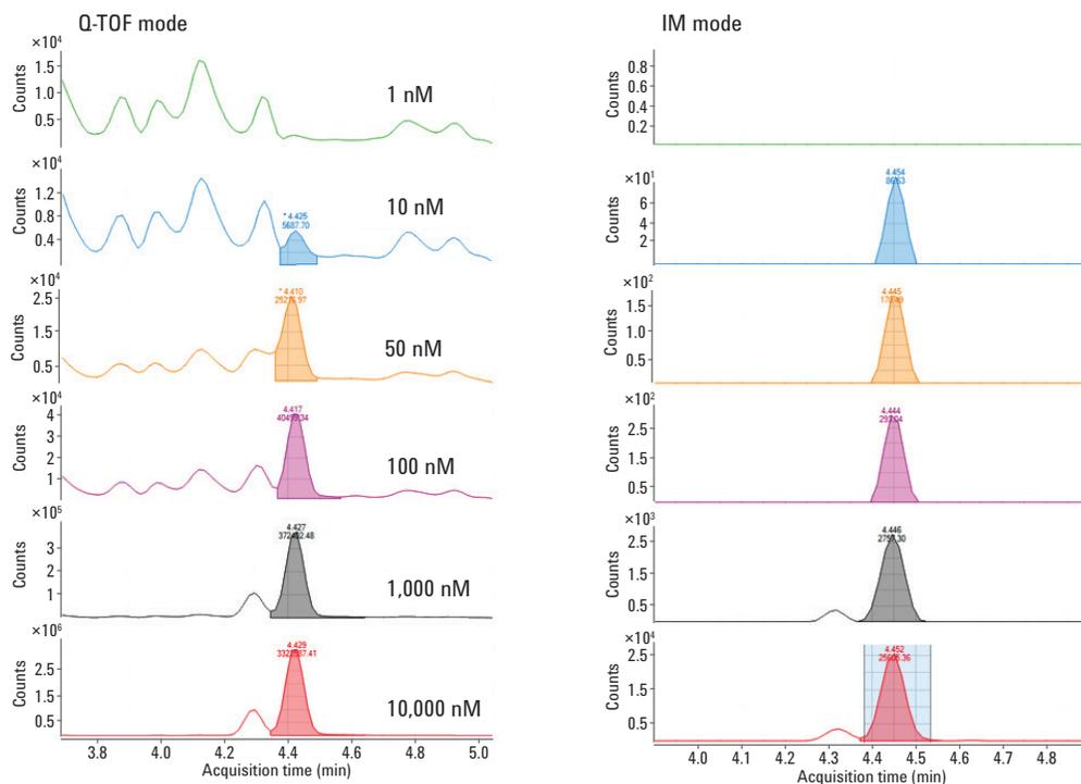
This example shows a comparison of detection limits between the Q-TOF and the IM Q-TOF modes of the system for a spiked compound (biological marker) in urine. Although very similar limit of detection (LOD) sensitivity is observed between these data acquisition modes, superior signal-to-noise (S/N) data using the IM-Q-TOF mode are obtained. Improvement in quantitative results are achieved due to the much lower background noise level.
