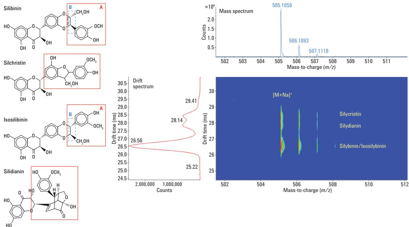
Silymarin, the active extract from plants, contains a mixture of flavonolignans consisting of silibinin, isosilibinin, silicristin, silidianin, and others. The most active compound in silymarin is silibinin. It has been extensively used in patients with liver disease. Ion mobility can be used to characterize these silymarin isomers. In this study, various isomers of silymarin are separated, and each of their unique collision cross-section values are determined (data not shown).
