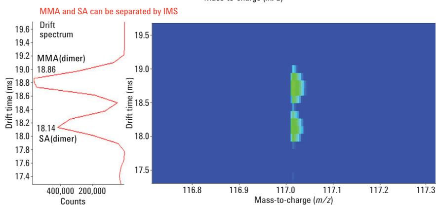
This is another example showing the ion mobility separation of the isomers of MMA, which is the vitamin B12 deficiency marker. In human plasma, its isomer (SA) is approximately 20 to 100x higher in concentration than MMA. These isomers are very difficult to separate by HPLC due to their polar properties. Our data demonstrate that the 6560 can resolve these isomers clearly, and the result can be used for accurate quantitation.
