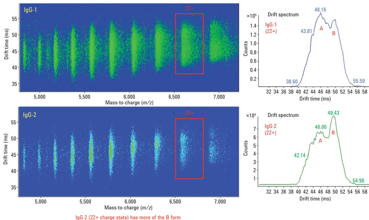
In this example, ion mobility is used to determine the relative amount of isoforms A and B in the IgG-1 and IgG-2 sample. In a side-by-side comparison, IgG-1 posts a slightly higher percentage of isoform A (native) than B at its 22+ charge state molecule. Conversely, a higher percentage of isoform B is detected in the IgG-2 sample.
