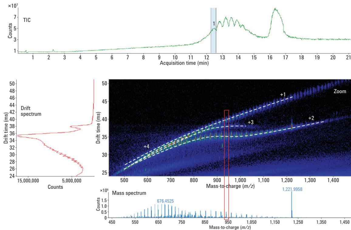
In this example, ion mobility is used to identify different hydrocarbon ion series in polymeric ink dispersants. The trend-lines illustrating the various charge-state hydrocarbon ion series are clearly resolved. In addition, the ion mobility specificity can significantly reduce the background matrix effect.
