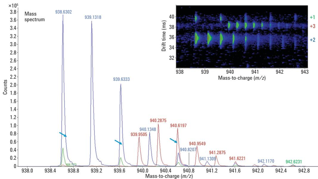
In this example, ion mobility is used to resolve overlapping charge-state isotopes that were unresolved by mass resolution only. This information is used to compare and confirm the quality level of the various ink products.
