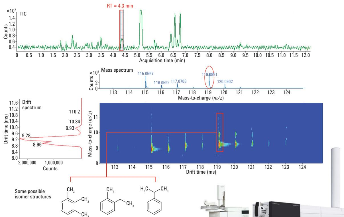
In this study, we use the GC-APCI interface coupled with ion mobility to analyze the ASTM standard compound mixture. For example, at the GC peak of 4.3 minutes, more than three separated compounds with many associated isomers in the mass range of 110 to 125 Da were found. Therefore, the Agilent 6560 provides higher peak capacity to successfully resolve the different isomers.
