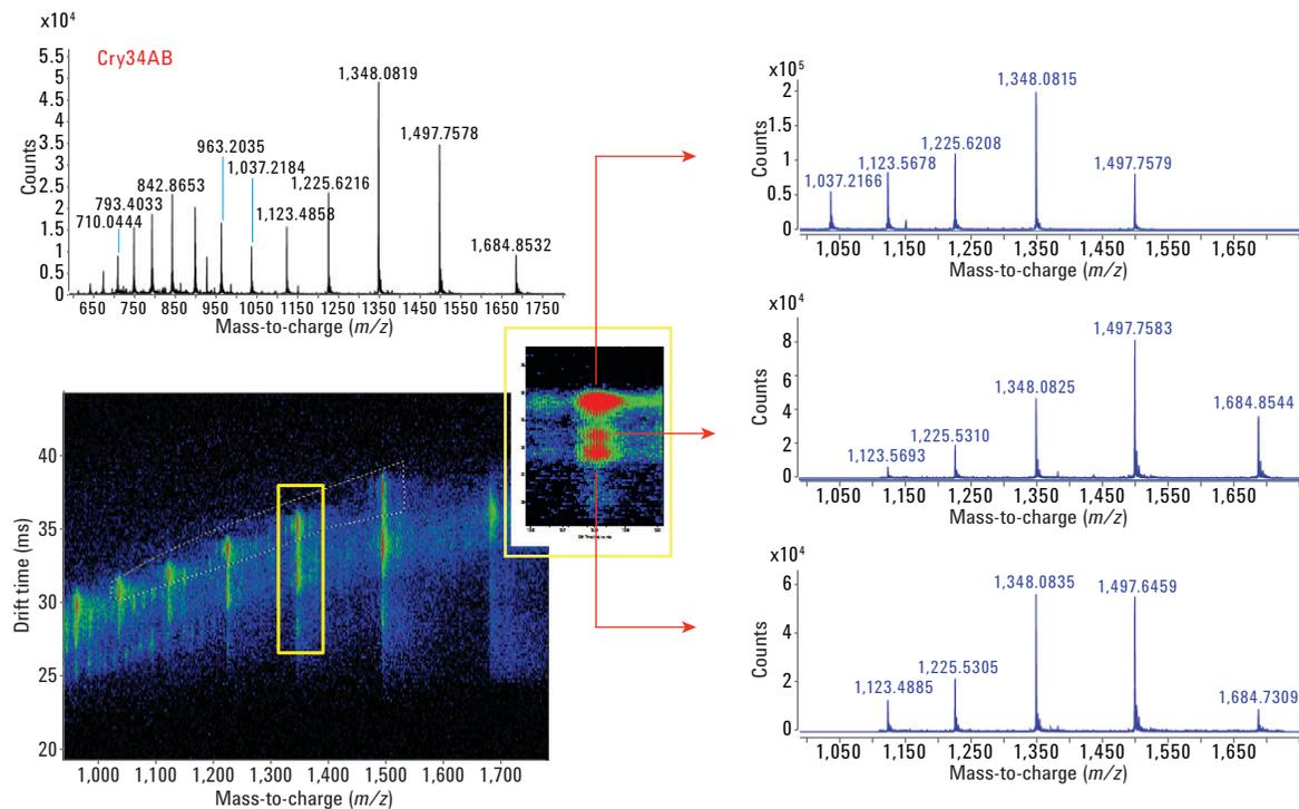
A protein sample (CRY34AB) under native and denaturing conditions is analyzed using ion mobility. Using just the IM information, it appears that there are possibly three isoforms, which are clearly separated. The IM results also confirm that the different isoforms generate different charge envelopes, indicating various protein folding structures, consistent with time-consuming X-ray crystallography.
