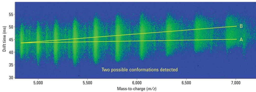
Two protein conformations are detected in the native IgG-1 sample using the 6560 system.
