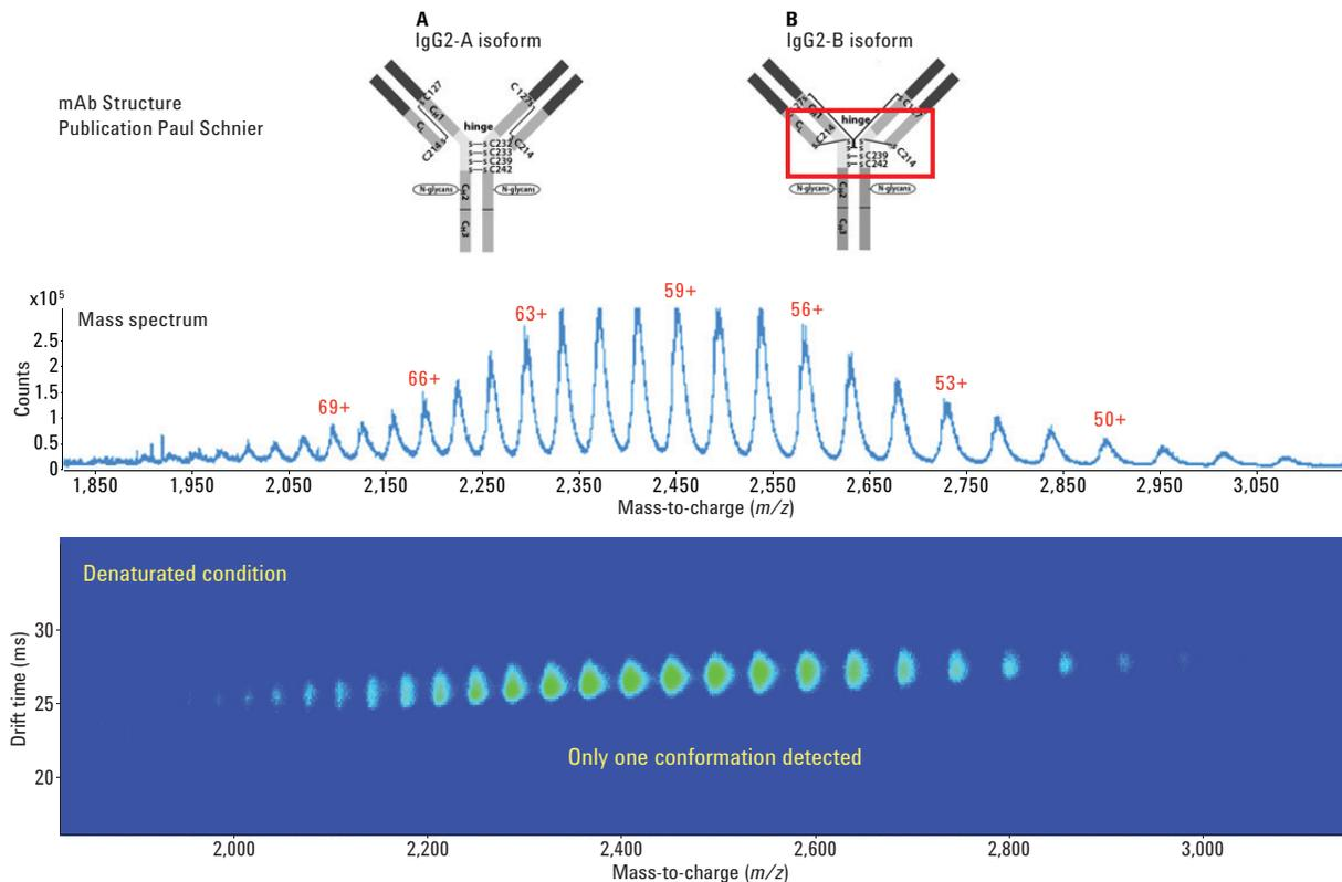
The IgG-2 molecule has two different conformations (isoforms A and B) under native conditions. However, normal LC/MS conditions, with a high content of organic solvent and 0.1% formic acid, will destroy the native structure. Only one denaturated protein conformation can then be detected.
