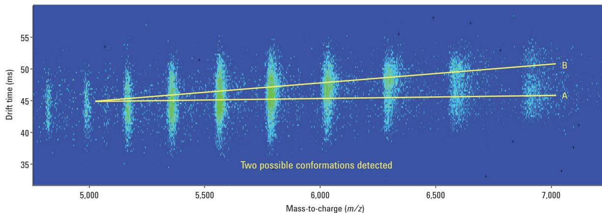
Under native conditions (100 mM ammonium acetate), the IgG-2 charge envelope will shift to higher  $m/z$  (5,000–7,000 range). Two protein conformations were clearly detected. Isoform A is the true native structure, and isoform B represents the IgG-2 with possible mismatch in disulfide bonds.
