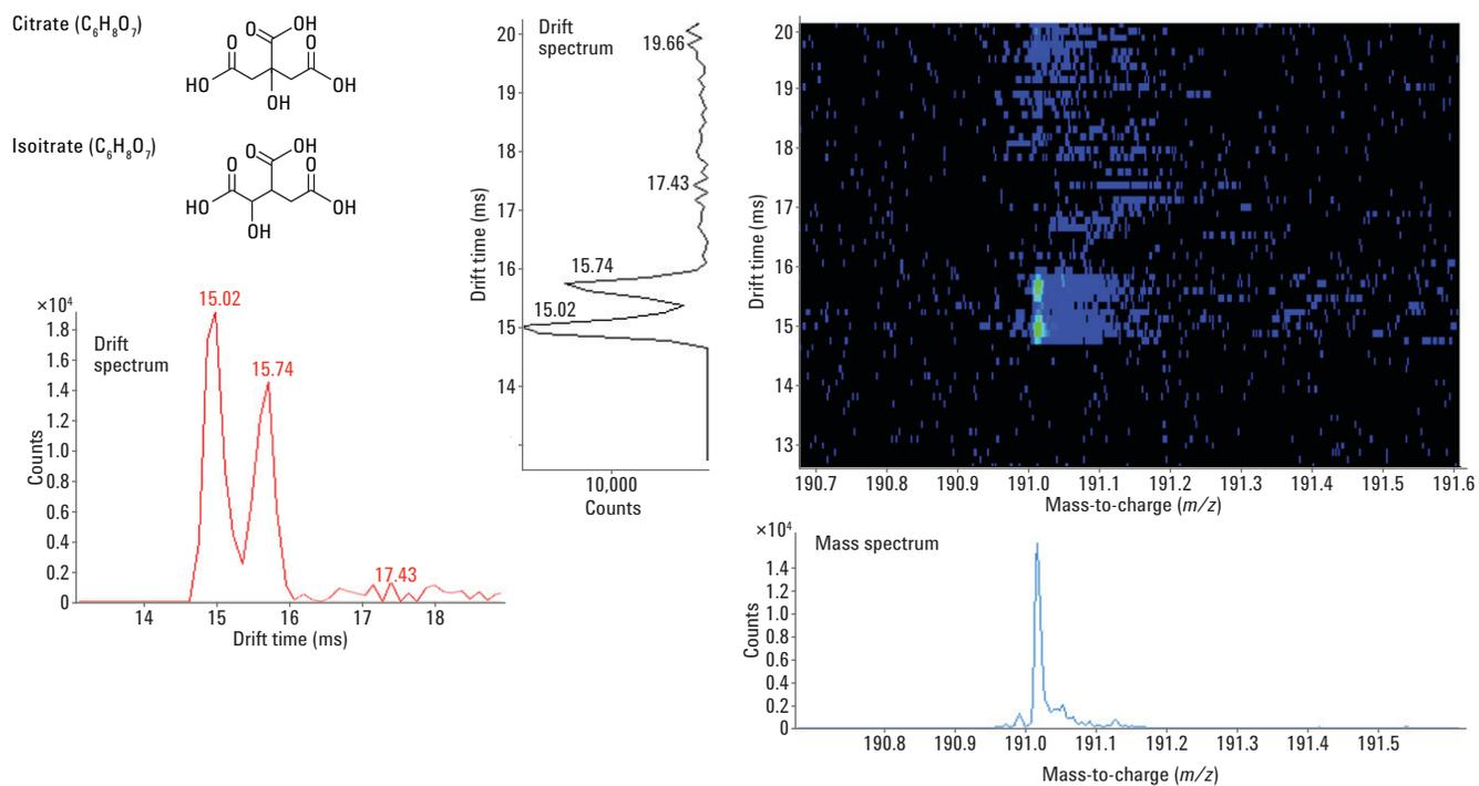
Citrate and isocitrate are isomers that are very similar in physical properties and structure. This presents challenges in their bio-analytical characterization. The Agilent 6560 Ion Mobility Q-TOF LC/MS shows clear resolution between these isomers.
