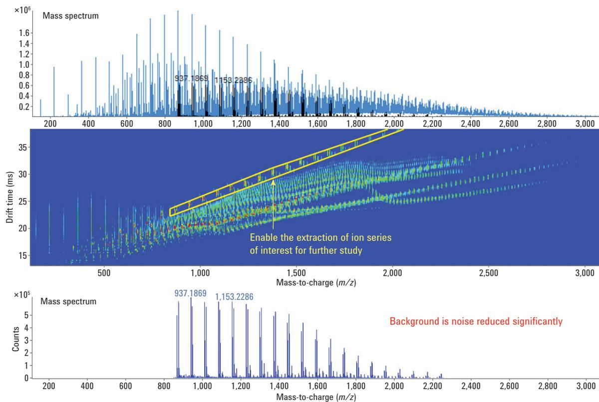
In this example, ion mobility is used to identify different hydrocarbon ion series in a diesel sample. The middle panel shows how ion mobility enables the extraction of ion series of interest for further study. The lower panel shows how ion mobility significantly reduces the background noise.
