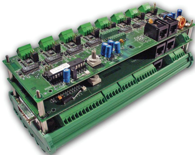
*Figure 3. Stackable extension boards - basic, analog, and digital*
