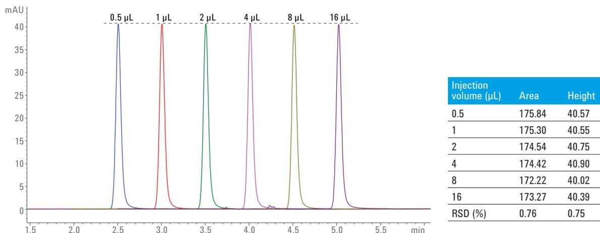
Figure 6. Injection volume linearity measurements using caffeine.
