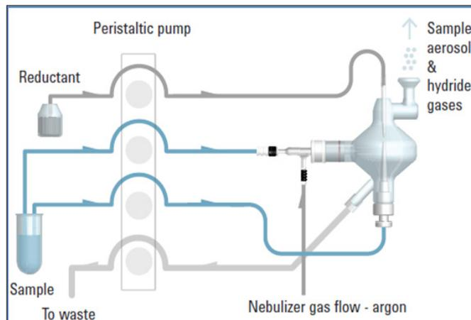
Figure 1. The Multimode Sample Introduction System (MSIS) operation
