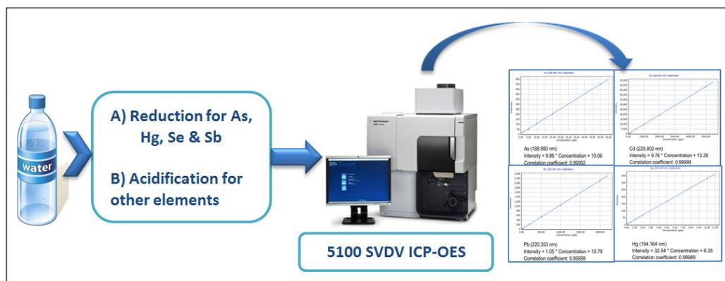
Figure 2. Schematic of water analysis workflow using the Agilent 5110 ICP-OES
