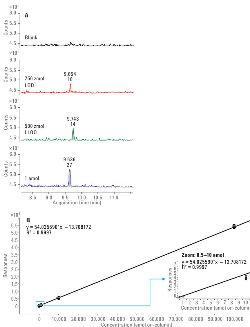
Figure 2. Nanoflow LC/MS results for the peptide standard LVNEVTEFAK in 10 fmol/ $\mu$ L trypsinized enolase. A) Stacked extracted ion chromatograms showing the LOD and LLOQ. B) Standard curve with inset showing detail for the range of the curve from 0.5 to 10 amol.
