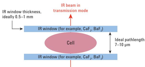
Figure 2 A schematic of the  $\text{CaF}_2$  cell used in this work for live imaging of *Micrasteris hardyi* cells.
