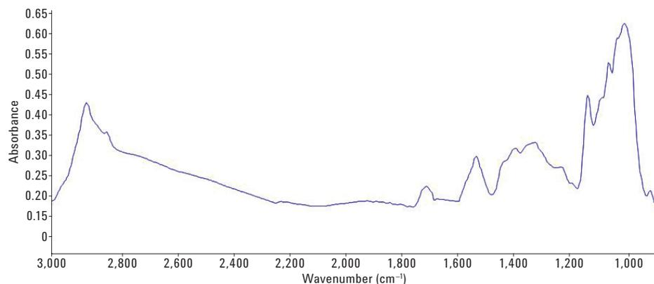
Figure 3. Mid-infrared spectrum of *Micrasteris hardyi* cells as measured in a  $\text{CaF}_2$  cell. Infrared bands arising from the specific chemicals contained in the cellular substructures are clearly observed. Spectral bands arising from aqueous background are mathematically eliminated.
