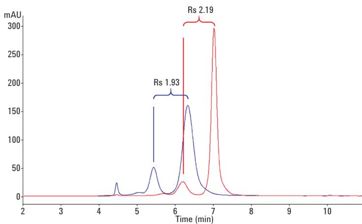
Figure 10B.  $\gamma$ -Globulin and BSA on an Agilent AdvanceBio SEC 300Å column using PBS, pH 7.4.
