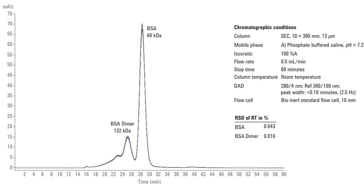
Figure 6. Low backpressure application: separation of bovine serum albumin (BSA) at 21 bar.
