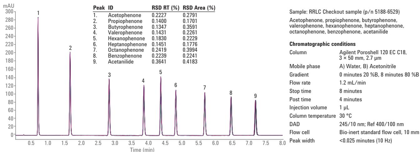
Figure 7. Area precision for conventional gradient runs for 1 and 0.5 µL.
