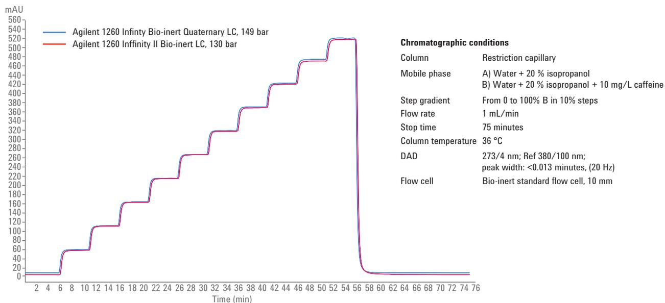
Figure 5. Overlay of step gradients. Agilent 1260 Infinity Bio-inert Quaternary LC and an Agilent 1260 Infinity II Bio-inert LC.
