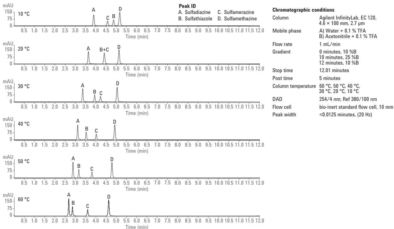
Figure 13. Thermosensitive sulfa drugs, with column temperature regulated through the bio-inert heat exchanger.
