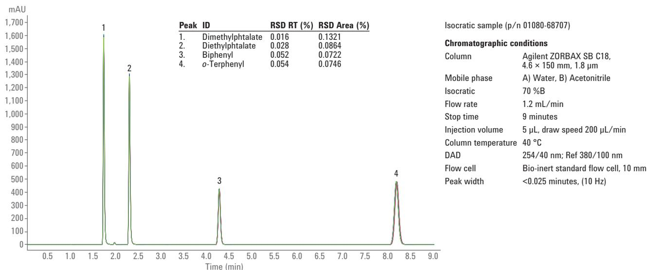
Figure 4. RT precision for conventional isocratic runs.
