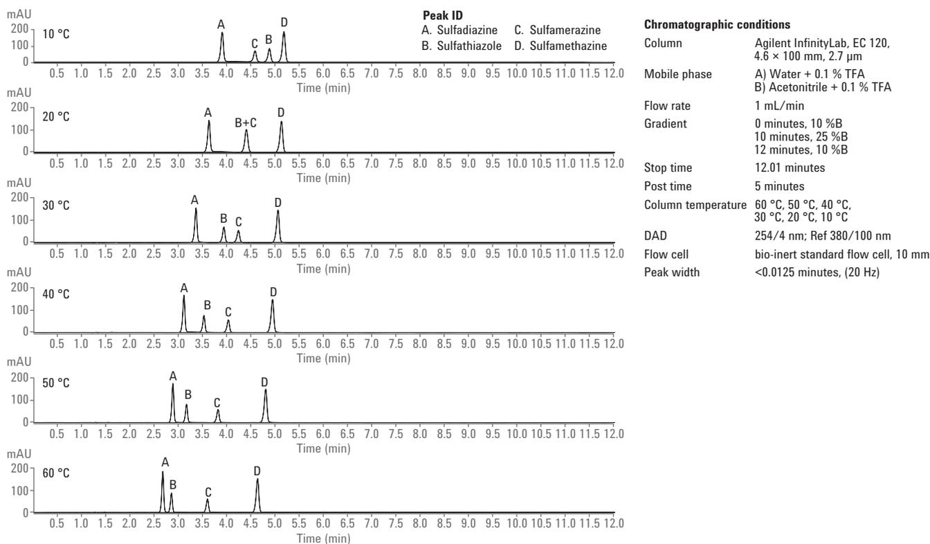
Figure 12. Thermosensitive sulfa drugs, with column temperature regulated through the standard heat exchanger.
