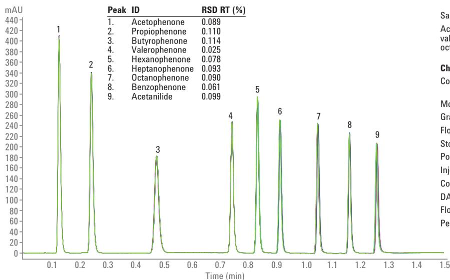
Figure 3. Precision of RTs for fast gradient runs.
