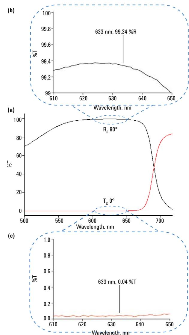
**Figure 4.** (a) Transmission and reflection spectra for s-polarized light measured on a CBS sample in the Cary 7000 UMS. (b) Reflection spectrum zoomed in around 633 nm. (c) Transmission spectrum zoomed in around 633 nm.
