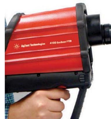
Figure 1. Agilent 4100 ExoScan FTIR spectrometer equipped with diffuse reflectance sample interface for measurement of composites
