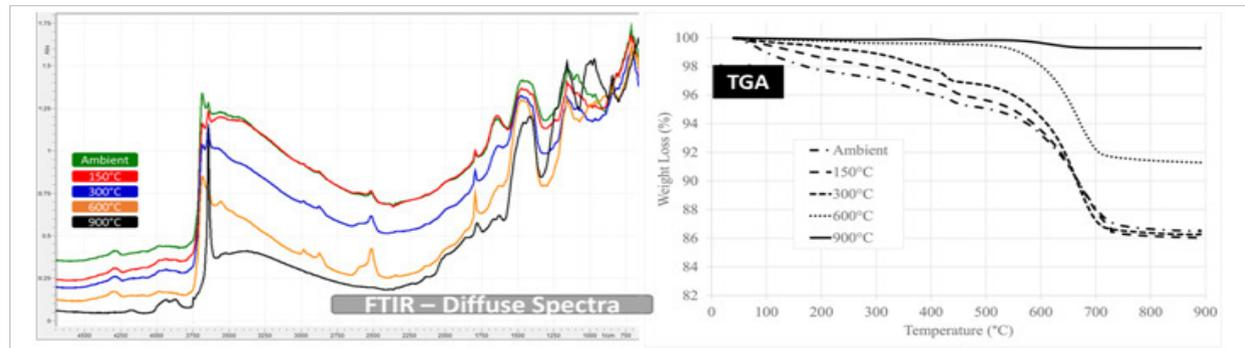
**Figure 6.** Left – diffuse spectra changes in a CEM I type concrete with gabbro rock aggregates at a variety of thermal treatments. Right the corresponding mass loss events for each concrete block post-thermal treatment.
