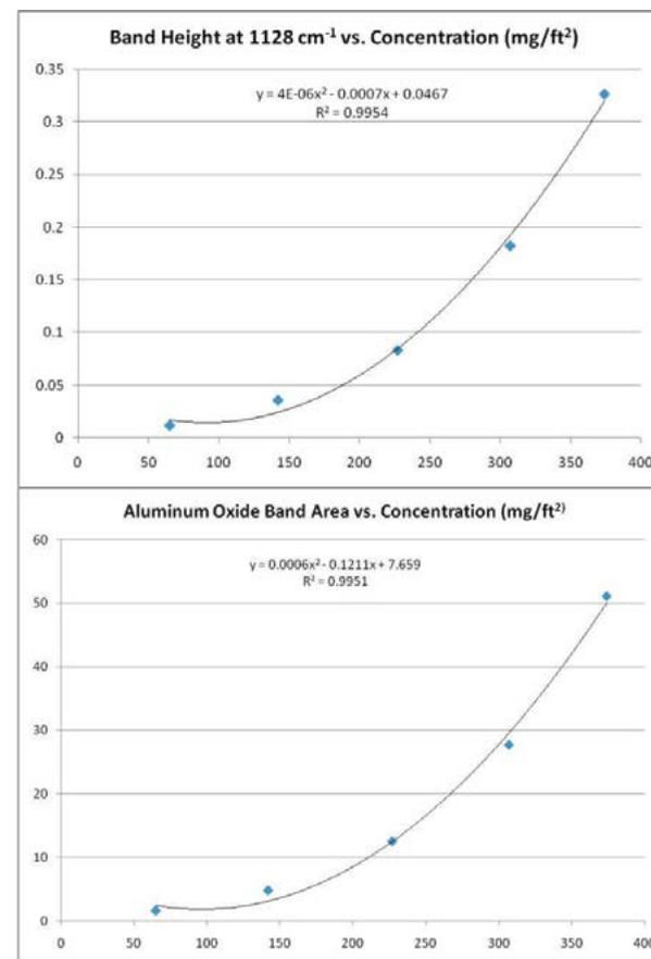
**Figure 2.** Calibration curves showing the aluminum oxide band height at 1128 cm<sup>-1</sup> versus concentration (top) and the aluminum oxide band area from 1390 cm<sup>-1</sup> to 995 cm<sup>-1</sup> versus concentration (bottom). Both calibration curves are fit by a quadratic equation with an excellent correlation coefficient.
