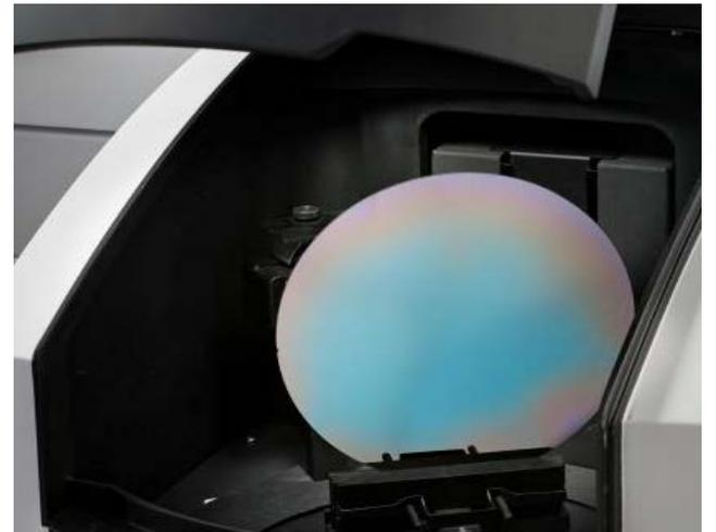
The unique sample handling capabilities of the Cary UV-Vis-NIR UMS instrument allow you to mount samples up to 200 mm in diameter in the sample compartment. The motorized sample stage moves the sample into position – allowing measurements at any position on the sample.
