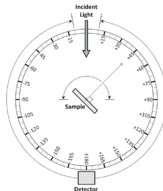
**Figure 1.** The AOI on the sample and the detector position can be set independently with  $0.02^\circ$  resolution. The AOI on the sample ranges from  $-85^\circ \leq \text{AOI} \leq 85^\circ$ . The detector can be placed at angles ranging from  $-10^\circ$  to  $10^\circ$ . As a result the Cary 7000 is able to determine R over the range  $5^\circ \leq |\text{AOI}| \leq 85^\circ$  and T over the range  $0^\circ \leq |\text{AOI}| \leq 85^\circ$ .
