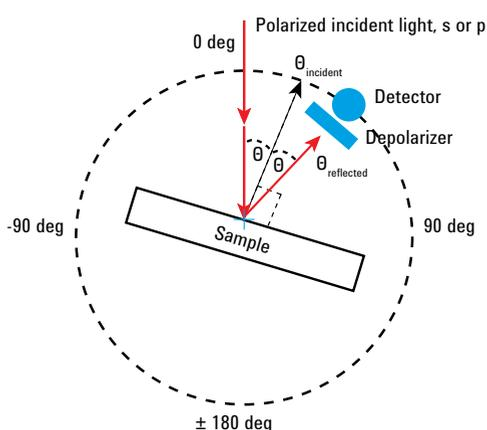
**Figure 3.** Schematic of the Cary 7000 UMS. Light incident onto the sample can be s, or p polarized. The detector module allows mounting of a depolarizer immediately before the detector. Absolute specular reflection of transmission can be measured
