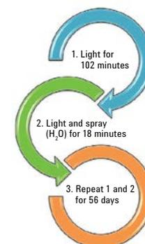
Figure 3. Two-step cycle used in the weathering process. The conditions are the environmental equivalent to sunlight at zenith at Florida's latitude and longitude. The acceleration of changes arises as the sun is not allowed to set for the whole test regime.
