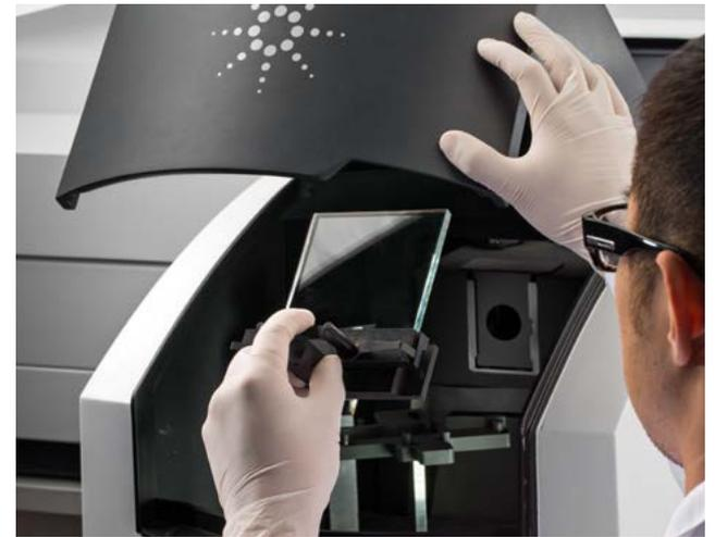
The revolutionary Agilent Cary 7000 Universal Measurement Spectrophotometer (UMS) can collect hundreds of UV-Vis-NIR spectra overnight, or characterize optical components or thin films in minutes to hours rather than hours to days.
