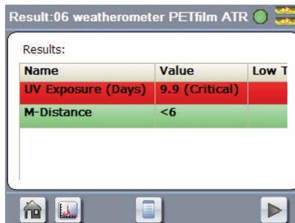
Figure 6. Results from this sample of PET indicate a significant degree of oxidation and alerts the user through a color coded (red) warning. The level for the warning, red critical value, can be tailored to suit.
