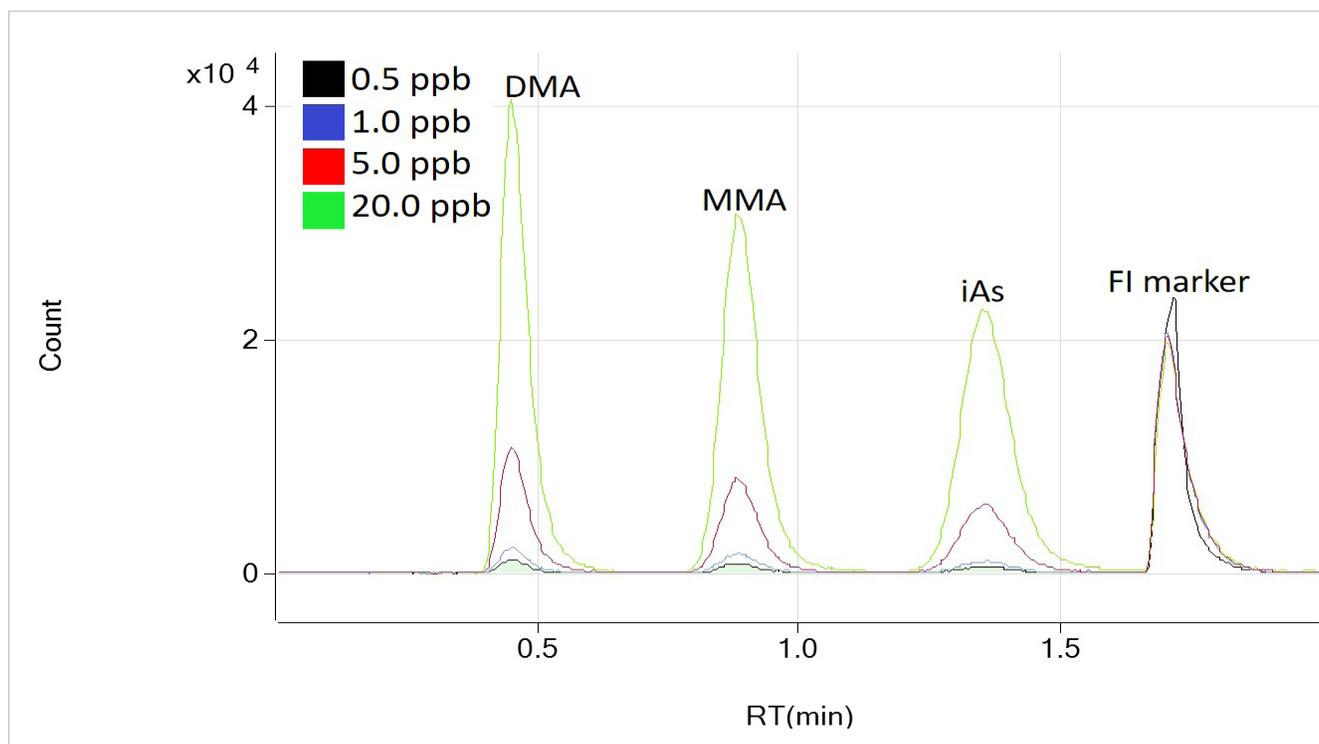
**Figure 1.** Overlay of the 0.5, 1.0, 5.0, and 20.0 µg/kg calibration standards. An AB internal standard (flow injection marker; fourth peak) was added post column via an external switching valve.
