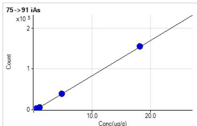
**Figure 2.** Calibration curves for DMA, MMA, and total iAs (sum of converted As(III) and As(V)).
