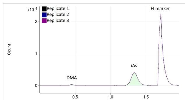
**Figure 3.** Chromatogram showing the overlay of the three replicates of wine sample V-1.
