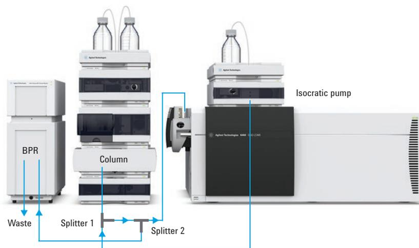
Figure 1. Configuration of the Agilent 1260 Infinity Analytical SFC System with the Agilent 6460 Triple Quadrupole LC/MS System. The column is connected directly to splitter 1 in the splitter assembly.
