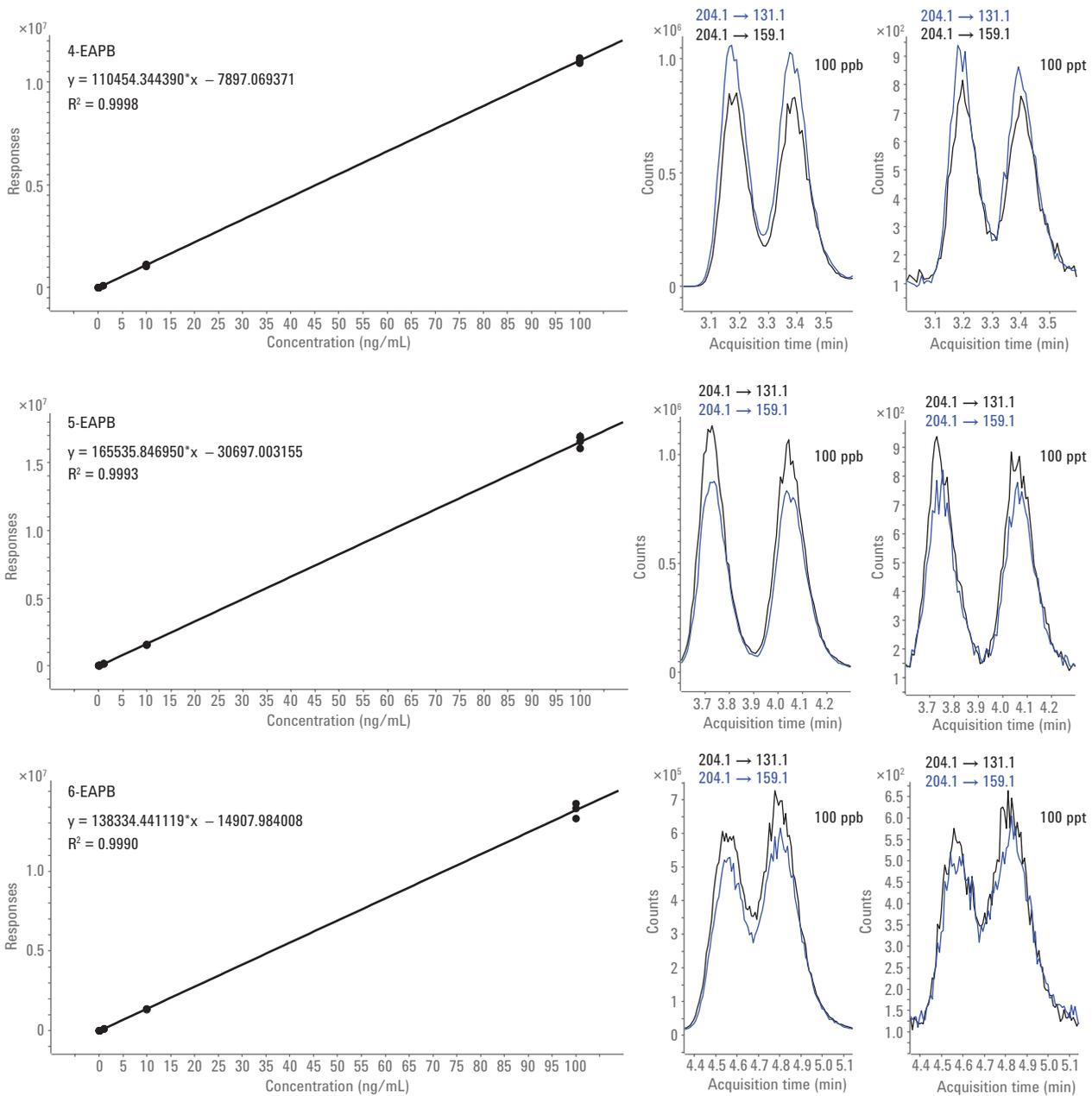
**Figure 7.** Calibration curves for 4-, 5-, and 6-EAPB between 100 ppt and 100 ppb. The quantifier and qualifier transition at 100 ppb and at 100 ppt (LOQ) are shown next to the individual calibration curves.
