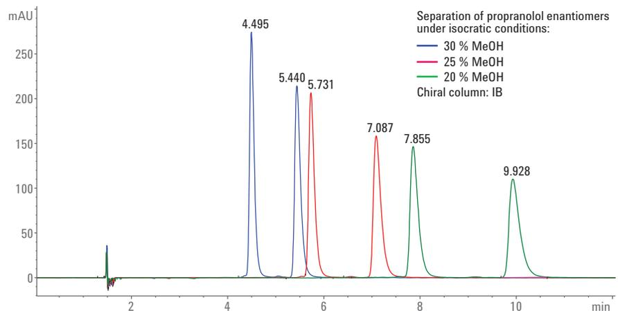
Figure 3. Separation of propranolol enantiomers on the chiral column IB with methanol as modifier.
