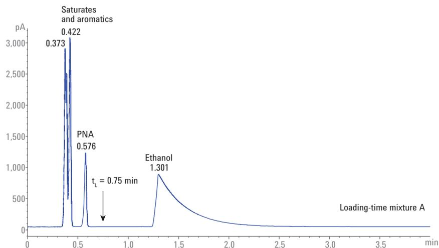
Figure 3. Determination of the sample loading time,  $t_L$ . Valves were switched to positions described in Figure 2B. Loading-time mixture A was used. The loading time  $t_L$  is determined when the aromatic and saturate compounds exit the PVA column, and the signal is back to baseline ( $t_L = 0.75$  minutes).
