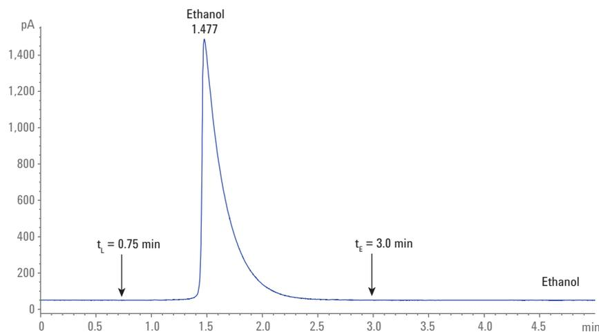
Figure 4. Determination of the backflush time for ethanol,  $t_E$ , after loading time,  $t_L$ . Ethanol was injected in valve position 2A, switching to position 2B ( $t_L = 0.75$  minutes). The backflush time  $t_E$  is determined when the ethanol peak returns to the baseline ( $t_E = 3.0$  minutes).
