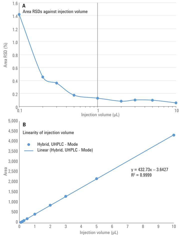
Figure 6. Performance in UHPLC mode. A) Determination of peak area RSDs in dependence of the injection volume (0.1, 0.2, 0.3, 0.5, 1.0, 2.0, 3.0, 5, and 10  $\mu\text{L}$ ). Area RSDs are typically below 0.2 % for all injection volume above 0.5  $\mu\text{L}$ . B) Peak area linearity of injection volumes between 0.1 and 10  $\mu\text{L}$ ,  $R^2 = 0.9999$ .
