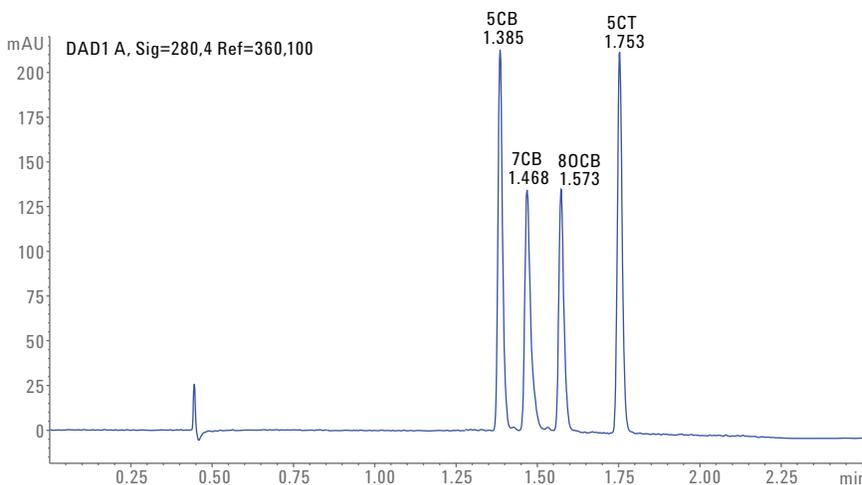
Figure 2. Separation of a mixture of liquid crystal compounds 5CB, 7CB, 8OCB, and 5CT using a fast gradient and within a short run time (50 μg/mL, each).
