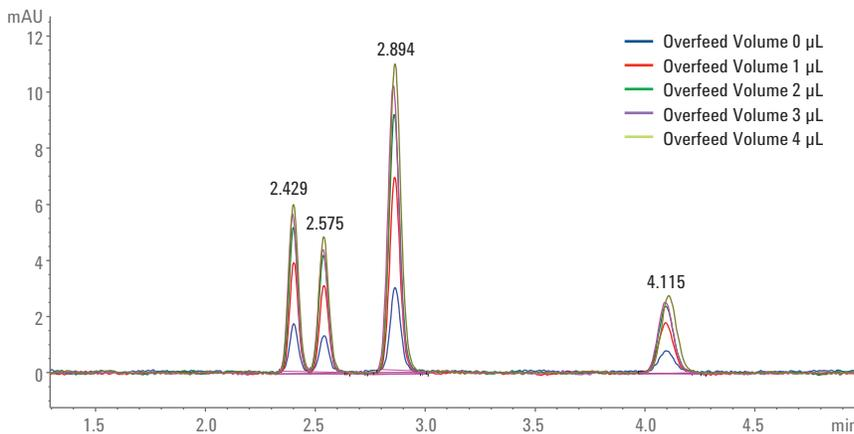
Figure 8. Influence of the Overfeed Volume on sample introduction for 0.1  $\mu\text{L}$  injection volume.
