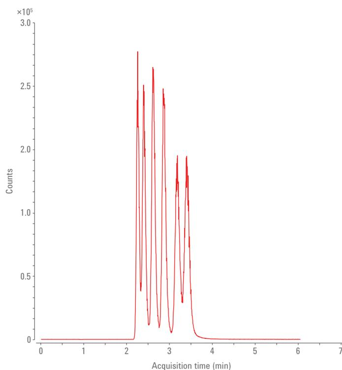
**Figure 4.** Method for the separation of all six isomers of 4-, 5-, and 6-EAPB with methanol as modifier.
