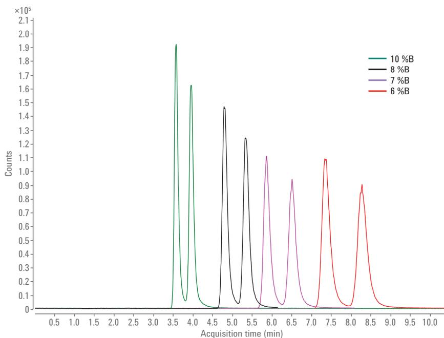
Figure 3. Chiral separation of D/L-amphetamine enantiomers (100 ppb) using different modifier content (modifier B: EtOH+ 0.1 % NH<sub>3</sub>(aq), flow rate: 3 mL/min, column temperature: 20 °C, column: CHIRALPAK AD-H 4.6 × 250 mm; 5 μm).
