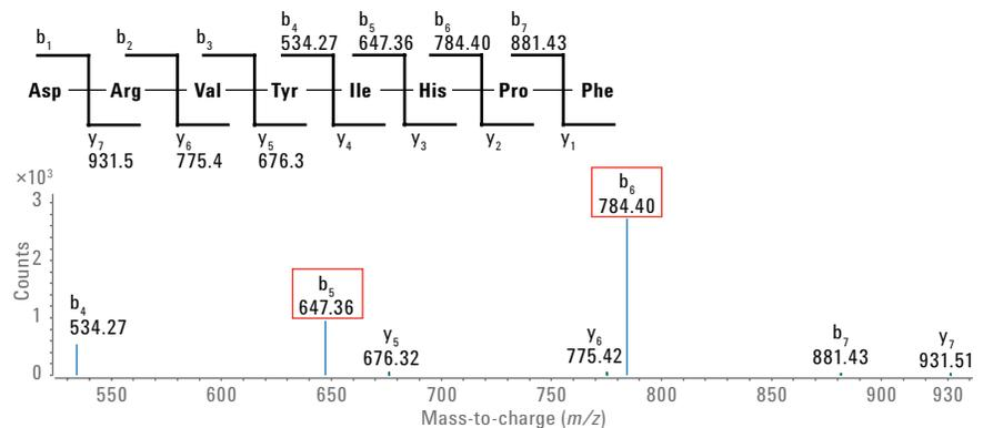
Figure 4. Fragmentation scheme of angiotensin II (MW = 1,046.2,  $[M+2H]^{2+} = 532.7$ ) and fragments identified from MS/MS spectra. The final DMRM and MRM method used the fragmentation  $532.7 \rightarrow 784.4$  and  $532.7 \rightarrow 647.3$ .
