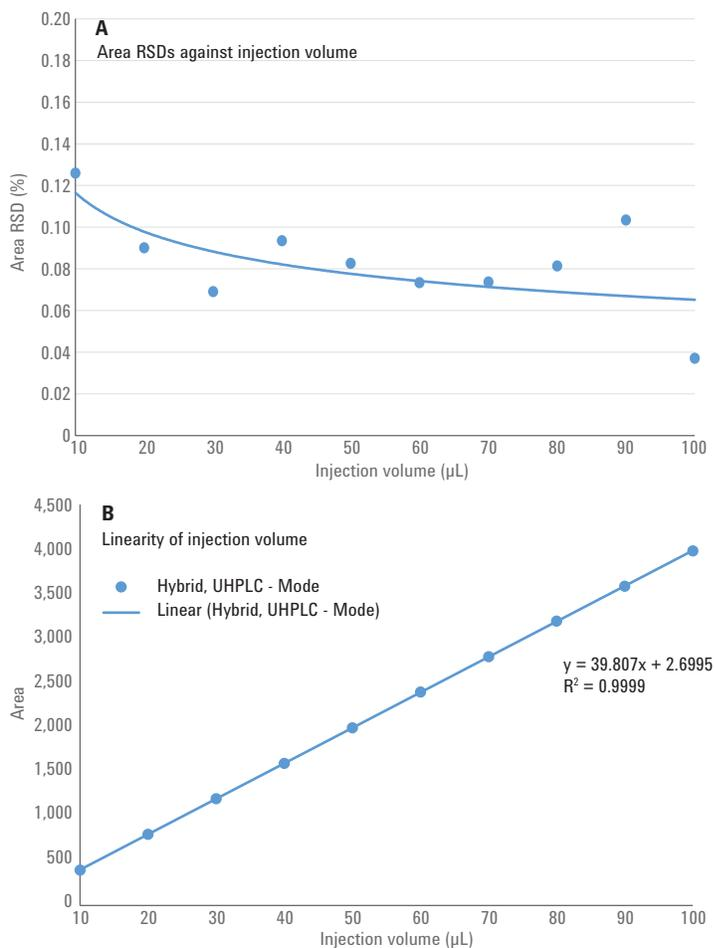
Figure 7. Performance in UHPLC mode for large injection volumes. A) Determination of peak area RSDs in dependence of the injection volume (10 to 100  $\mu\text{L}$ , step 10  $\mu\text{L}$ ). Area RSDs are typically below 0.12 %. B) Peak area linearity of injection volumes between 10 and 100  $\mu\text{L}$ ,  $R^2 = 0.9999$ .
