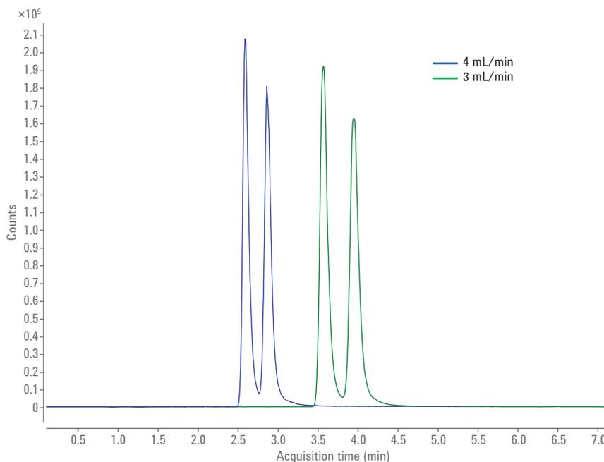
Figure 4. Chiral separation of D/L-amphetamine enantiomers (100 ppb) using different flow rates (modifier B: 10 % EtOH+ 0.1 %  $\text{NH}_3(\text{aq})$ , flow rate: 3 and 4 mL/min, column temperature: 20 °C, column: CHIRALPAK AD-H  $4.6 \times 250$  mm; 5  $\mu\text{m}$ ).
