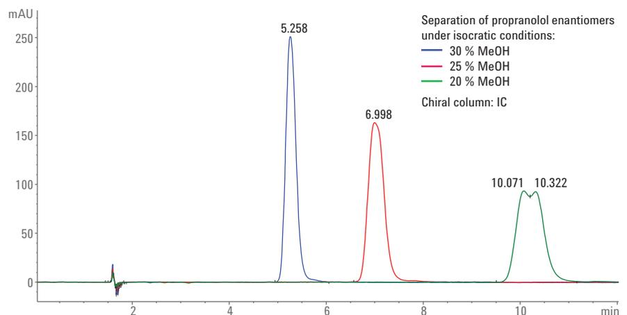
Figure 4. Separation of propranolol enantiomers on the chiral column IC with methanol as modifier.
