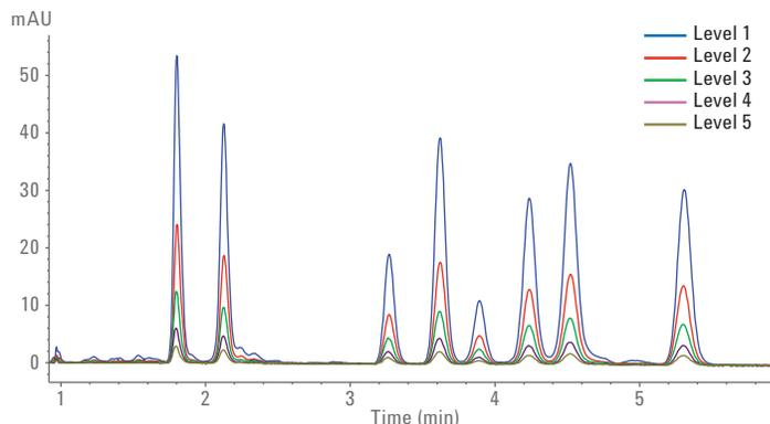
Figure 2. Overlay of calibration levels used to generate calibration curves for  $\alpha$ ,  $\beta$ ,  $\gamma$ ,  $\delta$ -tocopherol and  $\alpha$ ,  $\beta$ ,  $\gamma$ ,  $\delta$ -tocotrienol. (See Figure 1 for compound names, and Table 1 for the concentration of individual compounds and levels.)
