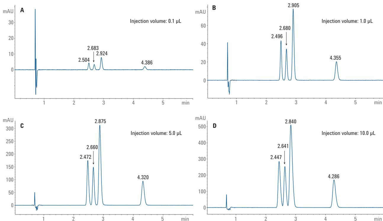
Figure 1. Different injection volumes at a Feed Speed of 400  $\mu\text{L}/\text{min}$ , and an Overfeed Volume of 4  $\mu\text{L}$ . A) 0.1  $\mu\text{L}$ , B) 1.0  $\mu\text{L}$ , C) 5.0  $\mu\text{L}$ , D) 10.0  $\mu\text{L}$ .
