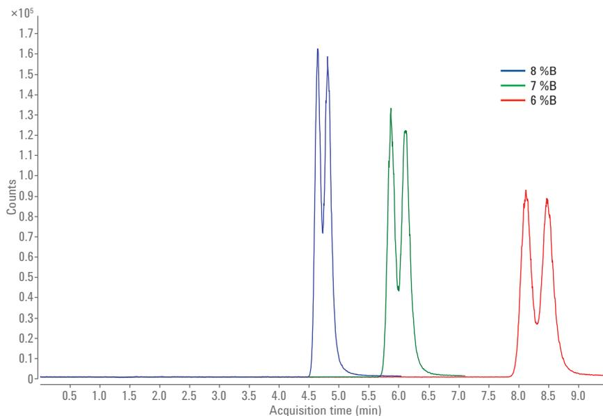
Figure 2. Chiral separation of D/L-amphetamine enantiomers (100 ppb) using different modifier content (modifier B: MeOH+ 0.1 % NH<sub>3</sub>(aq), flow rate: 3 mL/min, column temperature: 20 °C, column: CHIRALPAK AD-H 4.6 × 250 mm; 5 μm).
