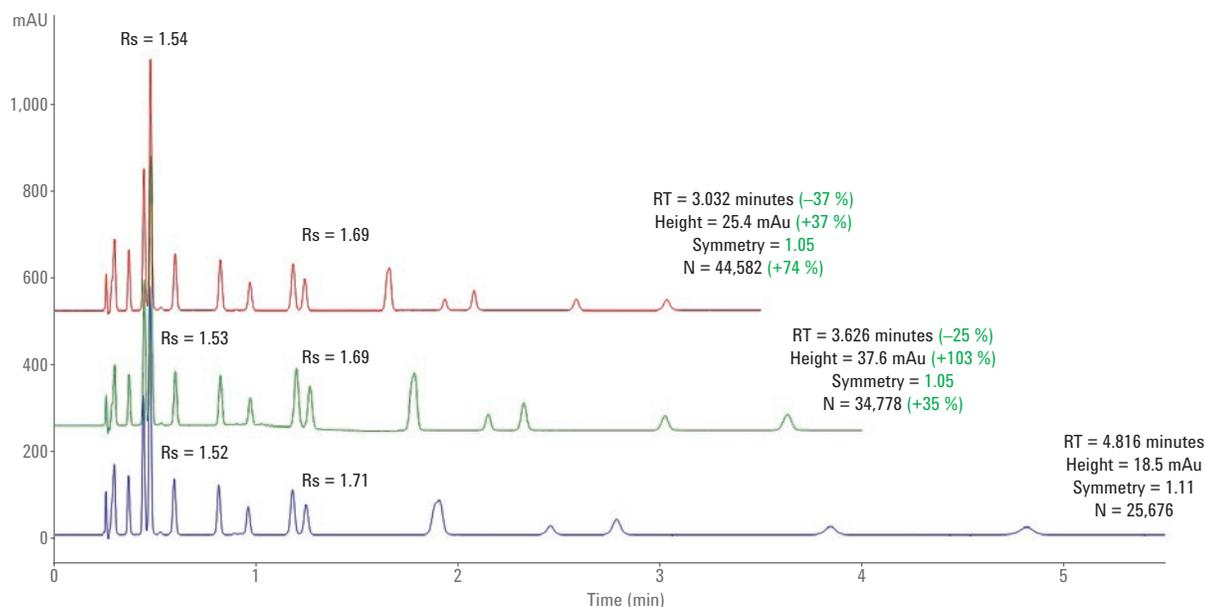
Figure 2. Comparison of the runs under isocratic conditions using pure CO<sub>2</sub>: The last peak eluted after 4.816 minutes with no focusing (blue), after 3.626 minutes when a backpressure gradient was applied (green), and 3.032 minutes when a flow gradient was used (red). In total, the run time could be reduced by 25 % with a backpressure gradient, and 37 % with a flow gradient.
