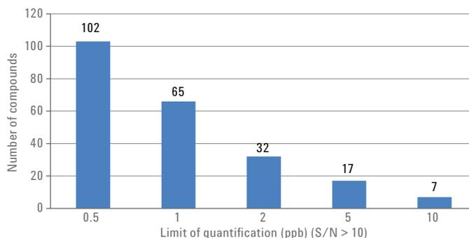
Figure 4. Distribution of LOQ for tested pesticides. There were 102 pesticides with a LOQ of 0.5 ppb, with an S/N > 10 and 167 had an LOQ of 1 ppb or lower. Only seven pesticides out of the 223 compounds had an LOQ of 10 ppb.
