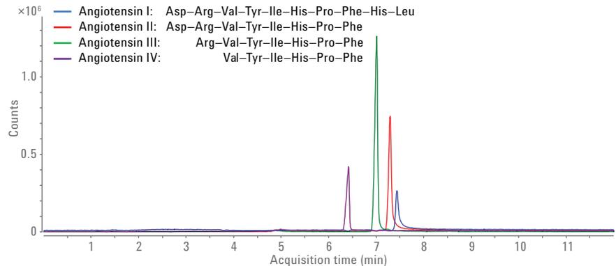
Figure 3. Separation of angiotensin I, II, III and IV by SFC (Gradient 1).
