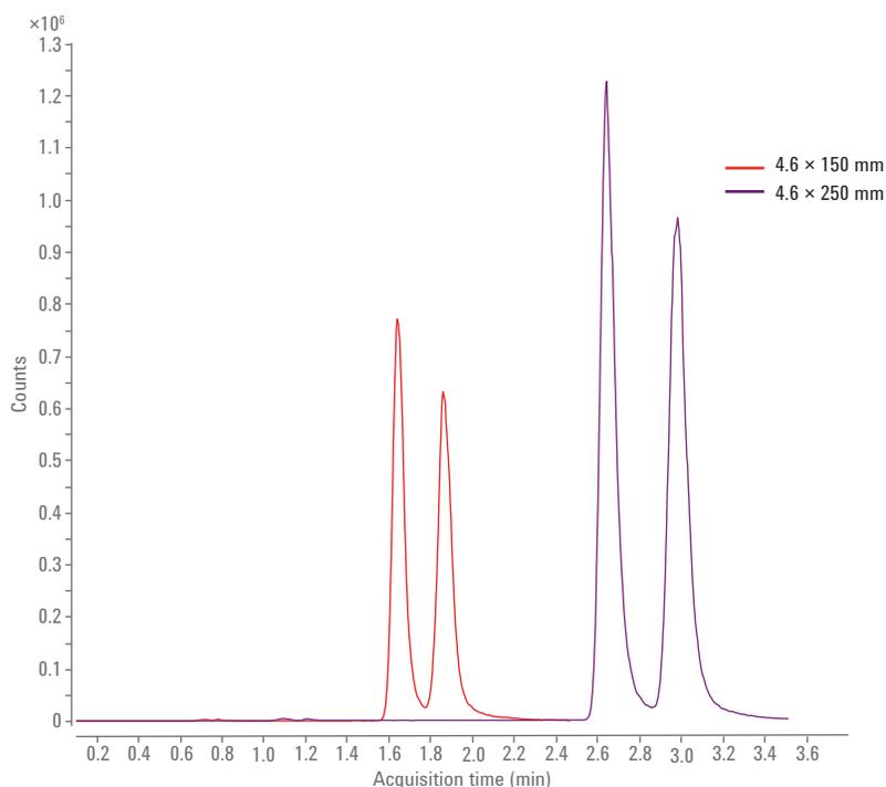
Figure 5. Chiral separation of D/L-amphetamine enantiomers (100 ppb) using different column sizes (modifier B: 10 % EtOH+ 0.1 %  $\text{NH}_3(\text{aq})$ , flow rate: 4 mL/min, column temperature: 20 °C, column: CHIRALPAK AD-H  $4.6 \times 250$  mm and  $4.6 \times 150$  mm, 5  $\mu\text{m}$ ).
