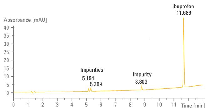
The 1220 Infinity II LC is ideal for the routine analysis of pharmaceutical preparations such as the quantification of the active ingredient ibuprofen and three earlier-eluting impurities.
