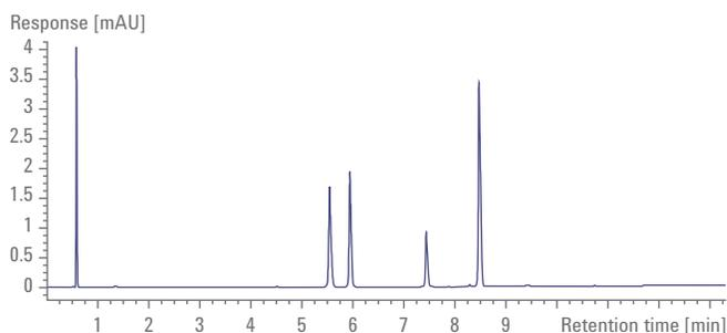
The 1260 Infinity II LC delivers robust separation and detection performance. In this example, 10 replicate analyses using an InfinityLab Poroshell 120 EC-C18, 3.0 x 150 mm, 2.7  $\mu$ m column achieve an RT RSD of 0.05 % at 5.53 min and 0.03 % at 8.46 min.
