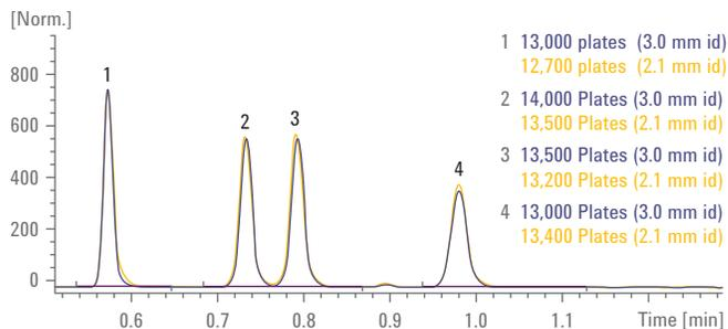
Thanks to lowest extracolumn volume the 1290 Infinity II LC achieves highest chromatographic efficiency in terms of plate numbers for both 2.1 mm and larger inner diameter columns.
