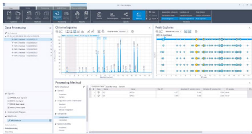
Peak Explorer helps you quickly identify samples with missing or extra peaks.
