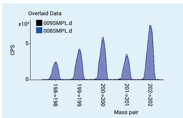
**Figure 1.** Hg isotopes with and without a W matrix, confirming the complete removal of W-based interferences by ICP-QQQ with MS/MS.
