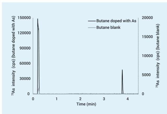
**Figure 3.** As chromatograms of doped liquefied butane and butane blank diluted 1:7.
