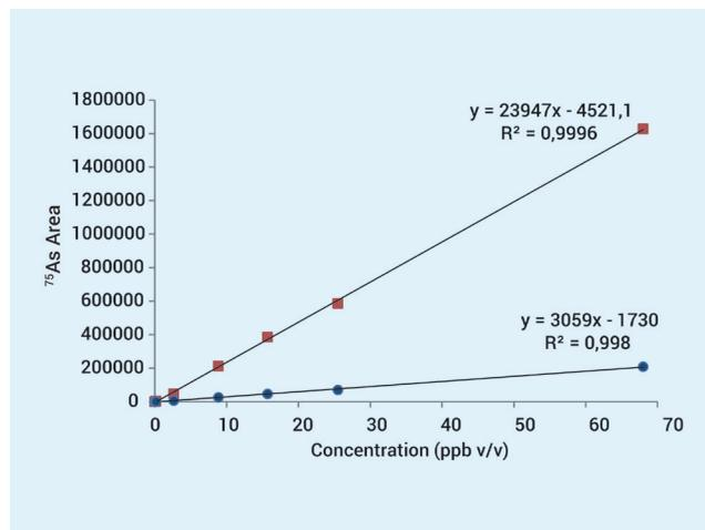
**Figure 2.** Calibration curves for “total As” (red points) and arsine (blue points) using arsine standards.
