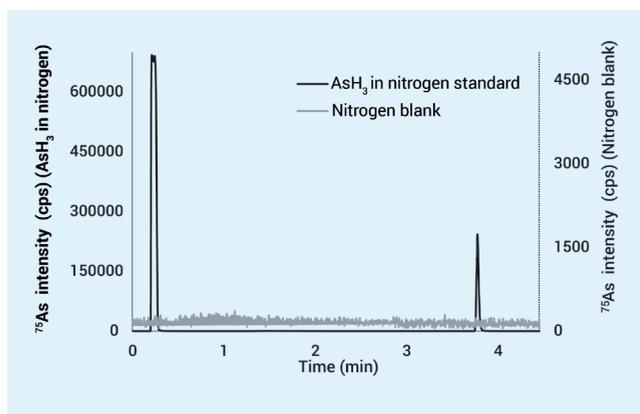
**Figure 1.** Chromatogram of arsine in nitrogen (68 ppb, v/v). (Reprinted with permission from Laura Freije-Carrelo et al, *Anal. Chem.*, 2017, 89 (11), pp 5719–5724. Copyright 2017 American Chemical Society).
