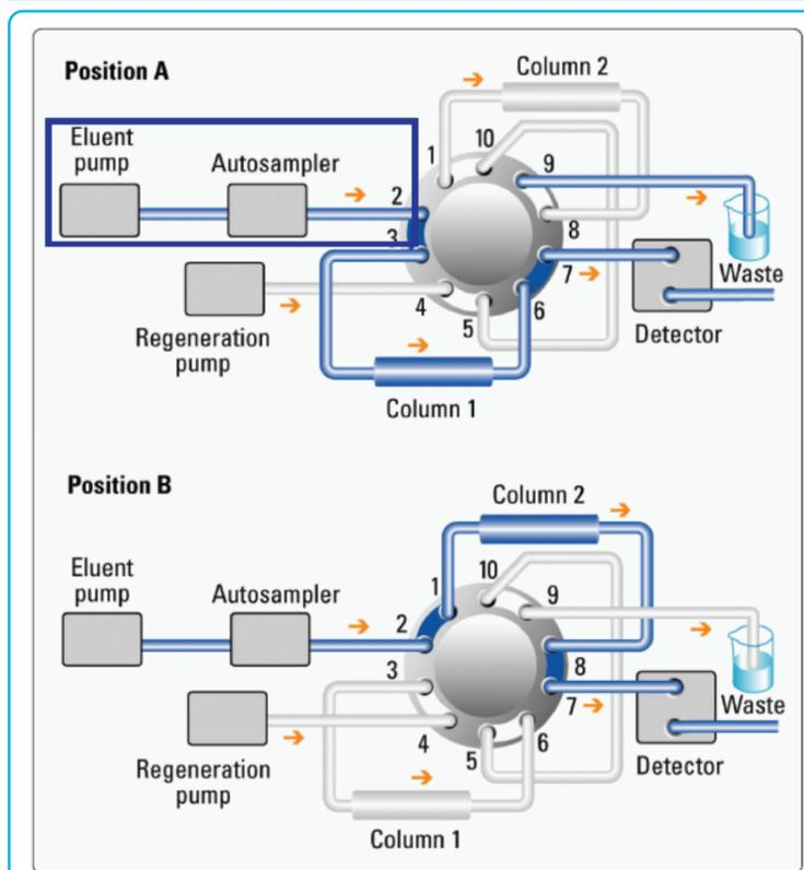
Figure 2. Alternating Column Regeneration valve configuration
