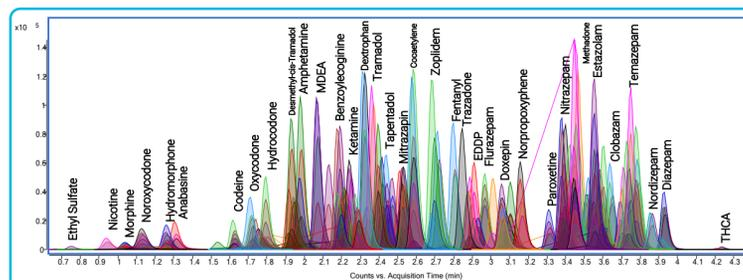
Figure 1. Example Chromatogram with 117 Analytes in 4.5 min
