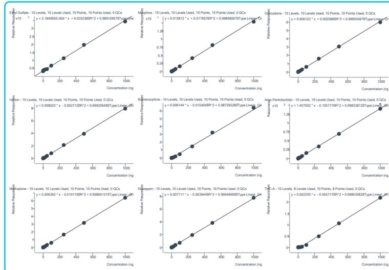
Figure 5. Examples of Quantitative Calibration Curves
