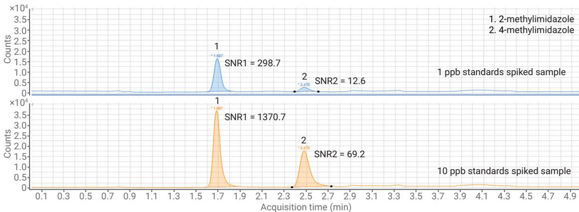
**Figure 3.** Chromatograms for 1 and 10 ppb standard spiked samples separated on an InfinityLab Poroshell 120 HILIC-OH5 column.
