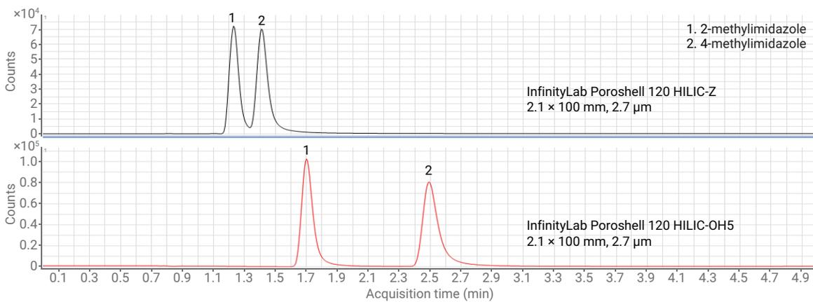
**Figure 2.** A comparison of the retention of 4-methylimidazole and 2-methylimidazole on an InfinityLab Poroshell 120 HILIC-Z and an InfinityLab Poroshell 120 HILIC-OH5 column with the same mobile phase.
