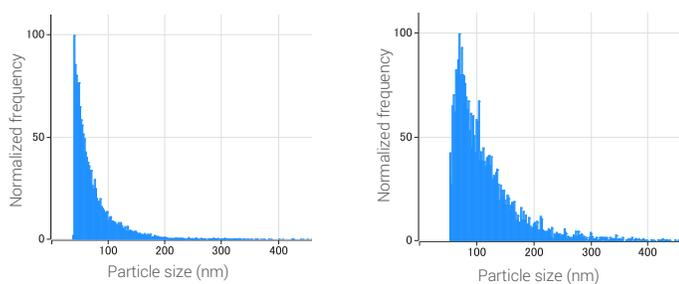
**Figure 3.** Particle size distribution of TiO<sub>2</sub> NPs (left) and ZnO NPs (right) in sunscreen C.
