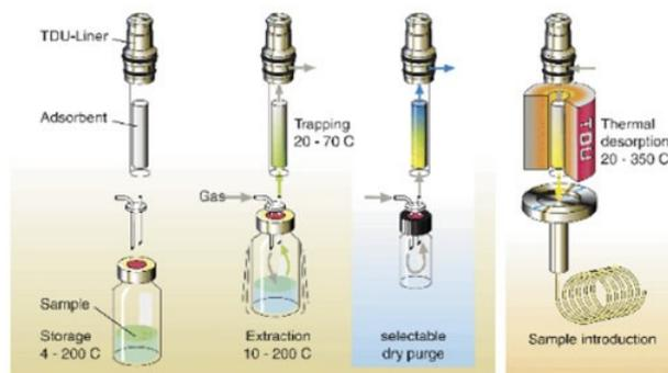
Figure 2 – Schematic view of the DHS Process
