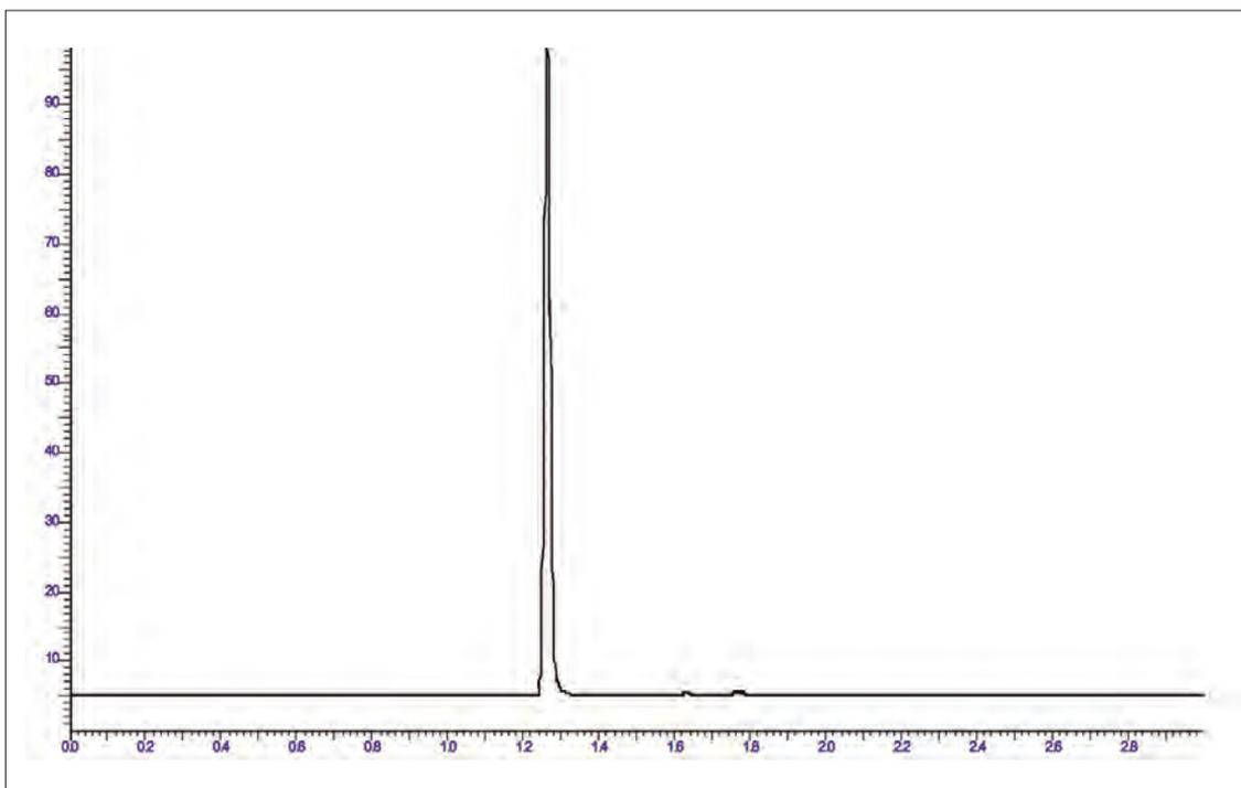
Figure 3. Chromatography demonstrating 0.1% methanol in a biodiesel matrix.
