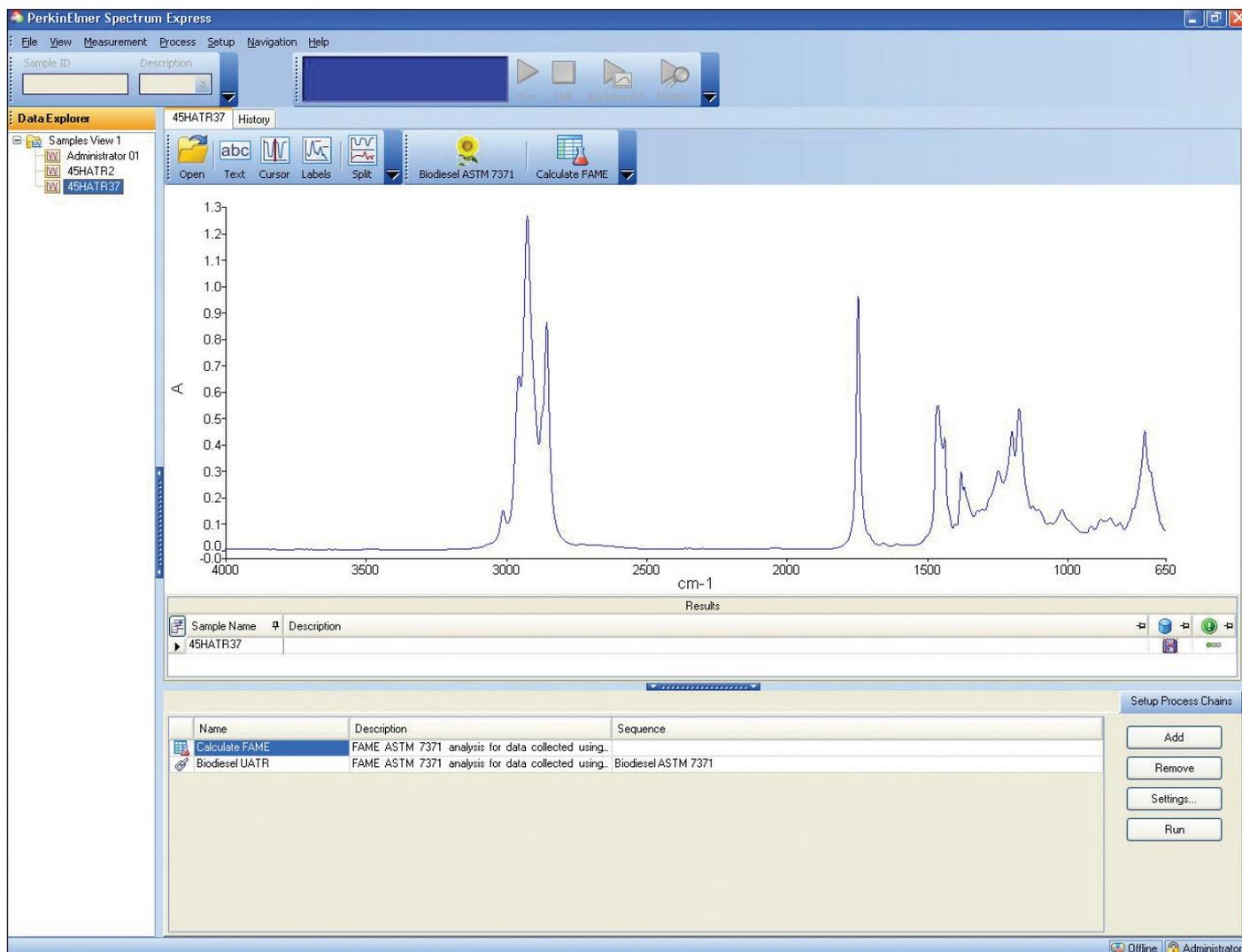
Figure 1. Spectrum Express biodiesel software and results table.
