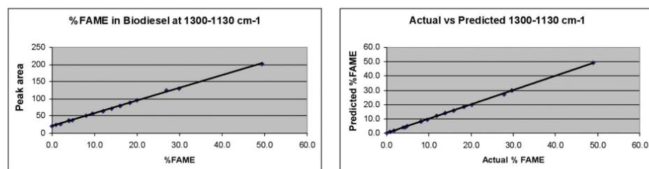
Figure 4: Beer's Law Calibration Method for 1300 – 1130 cm<sup>-1</sup>.
