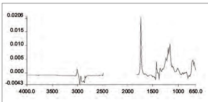
Figure 3. Biodiesel FAME concentration – PCR regression spectrum.
