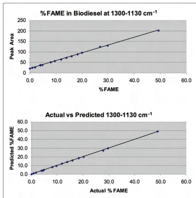
Figure 4. Beer's Law calibration method for 1300-1130  $\text{cm}^{-1}$ .
