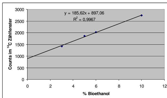
**Figure 7: Linearity of CPM measurements<sup>7)</sup>**
