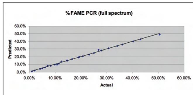
Figure 4. PCR calibration method.
