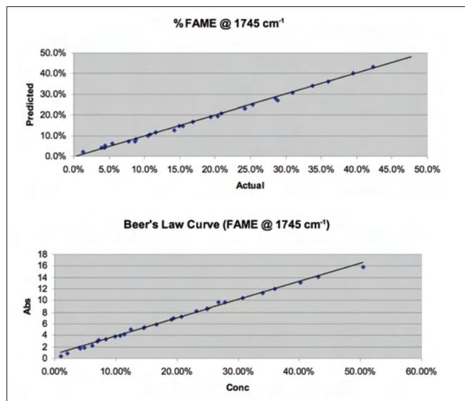
Figure 2. Beer's Law calibration method for 1745 cm<sup>-1</sup> peak.
