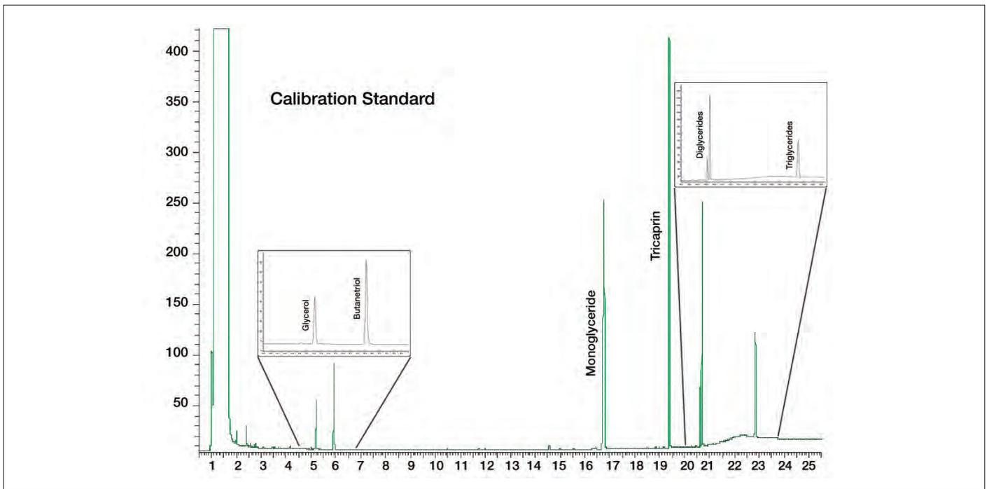
Figure 3. Free and total glycerol calibration standard.
