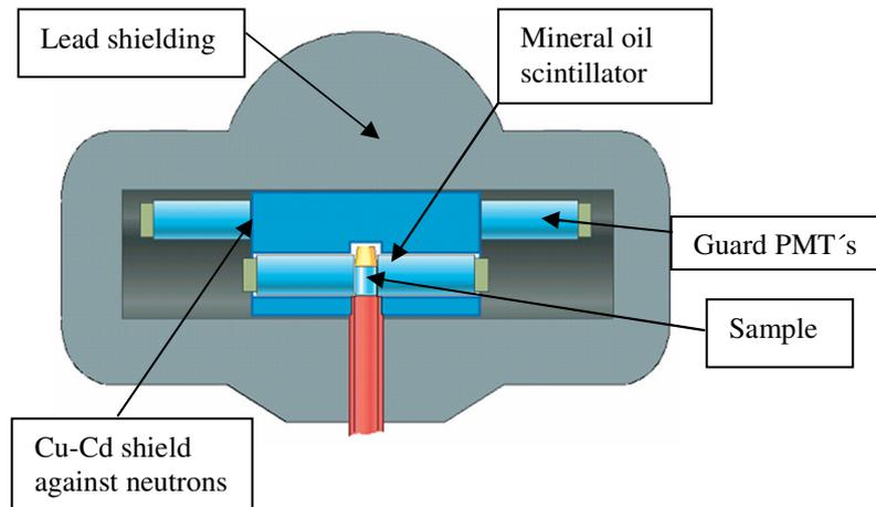
**Figure 3: Quantulus shielding and Guard-PMT's**
