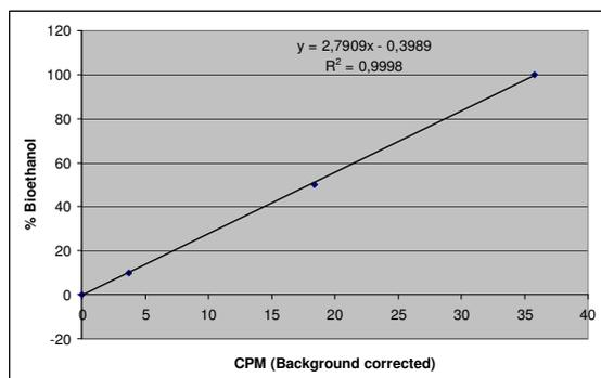
**Figure 8: Linearity of the CPM measurement<sup>15)</sup>**
