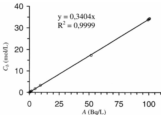
**Figure 10: Linearity of DPM measurements in the Quantulus<sup>6)</sup>**
