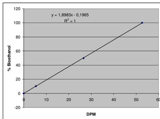
**Figure 9: Linearity of the DPM measurement<sup>15)</sup>**
