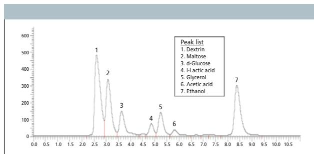
**Figure 1:** Actual 24-hour fermentation sample from ethanol production monitoring.
