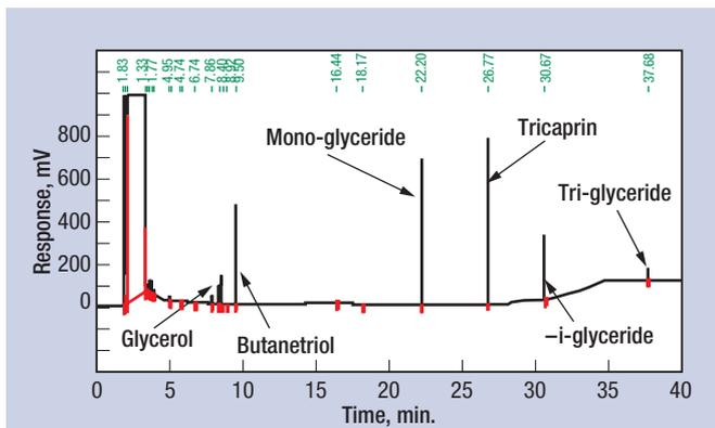
**FIG. 3** Chromatographic display of a calibration mixture of glycerol, mono-, di- and triglyceride and the internal standards butanetriol and tricaprin—generated using ASTM Method D-6584 (see Table 3 for concentration levels).
