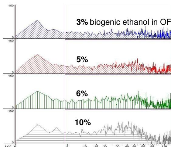
**Figure 6: <sup>14</sup>C spektra in Otto-fuel (OF) with different amounts of bioethanol.<sup>7)</sup>**
