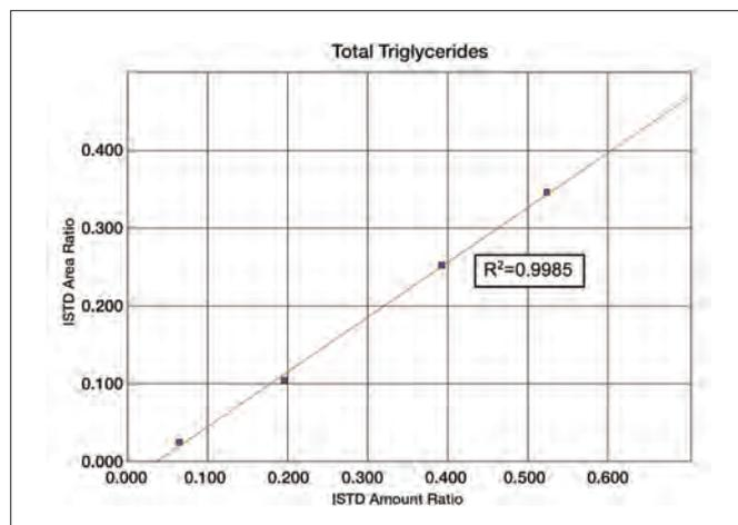
Figure 2. Example calibration plot for total triglycerides following EN 14105.
