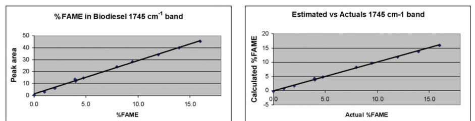
Figure 2: Beer's Law Calibration Method for 1745  $\text{cm}^{-1}$  Peak
