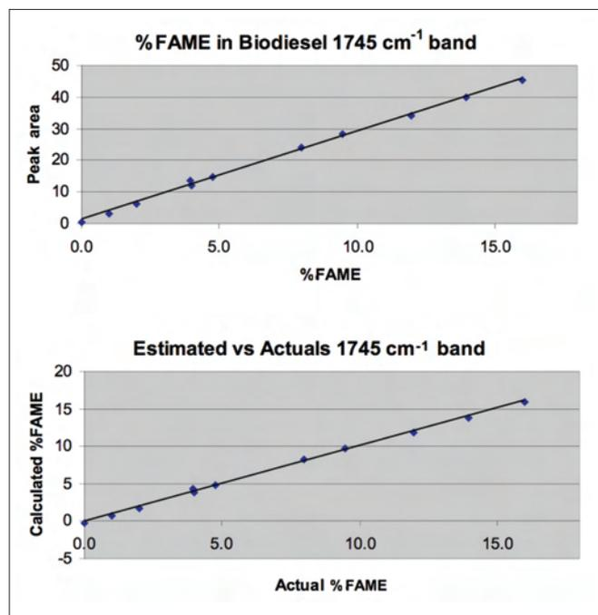
Figure 2. Beer's Law calibration method for 1745  $\text{cm}^{-1}$  peak.
