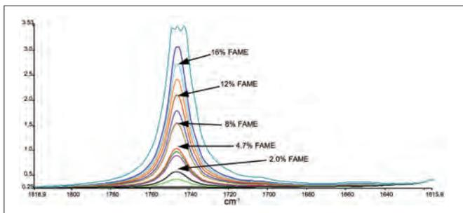
Figure 1. FT-IR spectra of varying FAME concentrations in diesel fuel.
