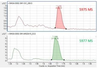
Figure 4: SIM chromatogram comparison between an Agilent MS 5975 and 5977 for bromomethane and chloroethane at 0.5 μg/l
