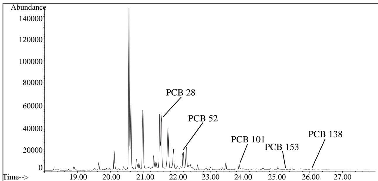
**Figure 6.** Selected ion chromatogram of the last filter layer, PCB traces.
