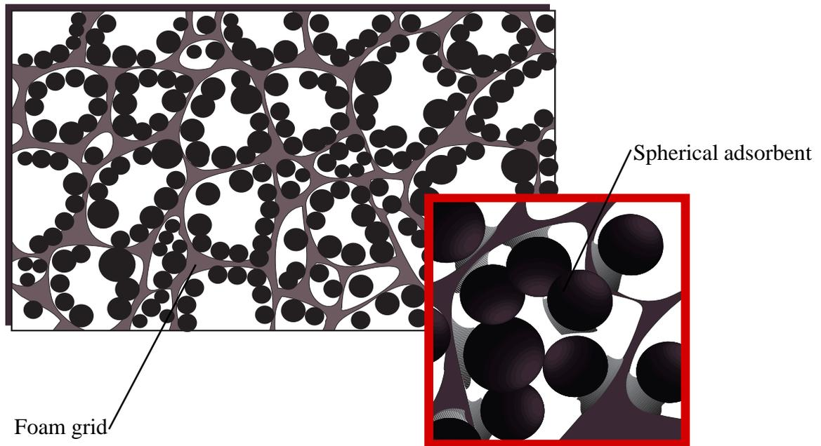
**Figure 1.** Construction of the open-porous NANOSORB™ filter.
