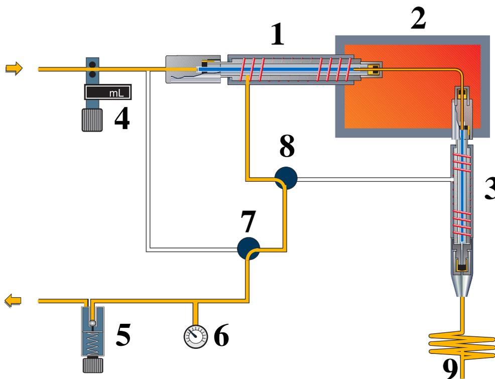
**Figure 4.** Schematic of the applied system which consists of a thermodesorption system (1), a temperature controlled transfer capillary (2), a cooled injection system (3), standard backpressure pneumatics with mass-flow controller (4), backpressure regulator (5), pressure gauge (6) and split/splitless valve (7), including an additional 3/2-way solenoid (8) to switch the splitflow between TDS and CIS. The analytical column (9) is directly connected to a mass selective detector.
