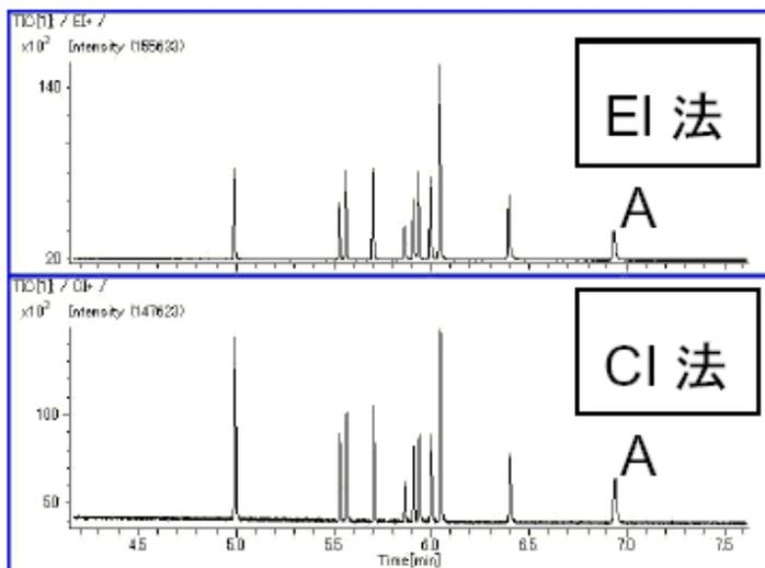
Figure 1. TIC of liquid crystal (top: EI; bottom: CI)
