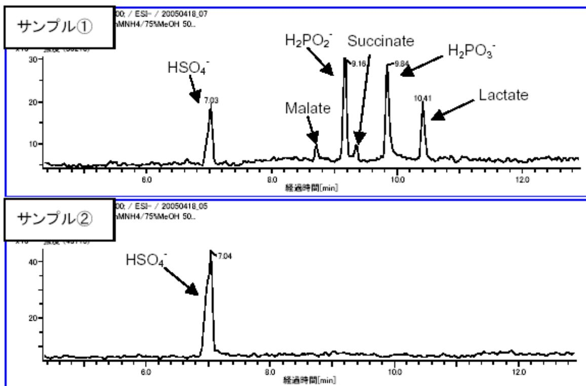
Figure 1. Mass electropherograms of anions in plating liquids (accumulated)
