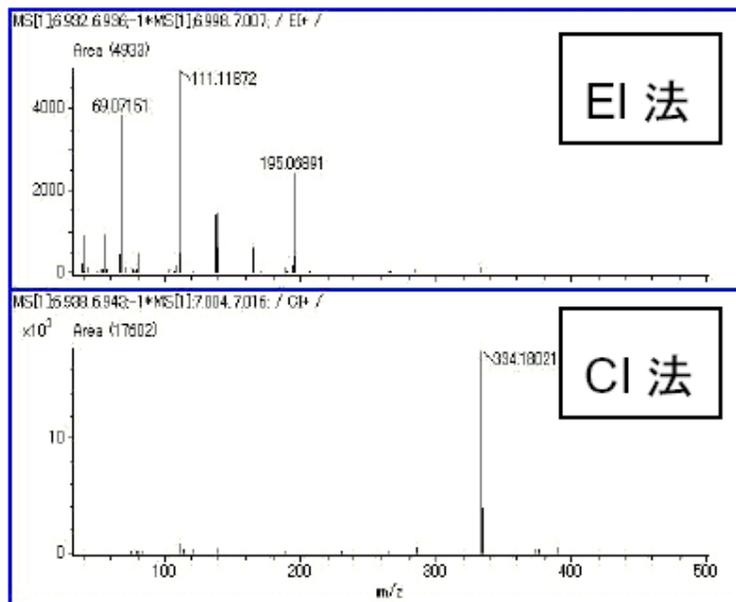
Figure 2. Mass spectra of Component A
