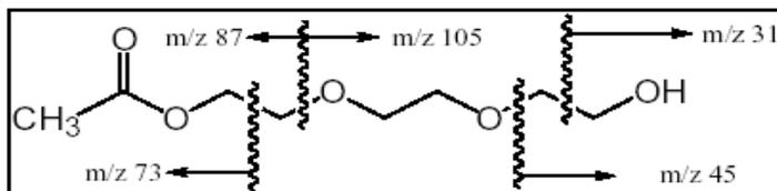
Figure 3. Estimated structure of unknown component in triethylene glycol
