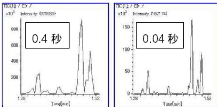
**Figure 2. Chromatogram peak analysis in fast GC at different recording speeds**
