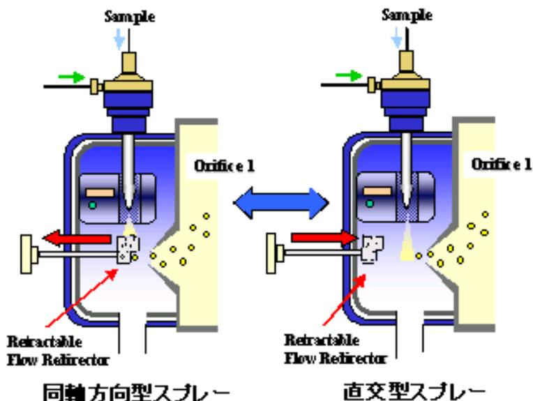
Vertical gas flows from the sprayer are effective in minimizing contamination buildup in the MS system. For some samples, however, ionization efficiency is often inferior to coaxial gas flows.
