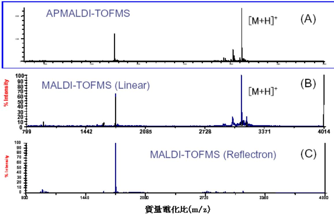
Figure 2. MS spectra of  $\beta$ -casein ( bovine ) fragment 1-25 acquired in AP MALDI-TOFMS (A), Linear mode of MALDI (B), and Reflectron mode of MALDI (C)
