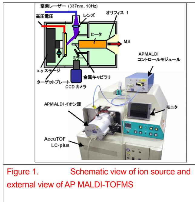
Figure 1. Schematic view of ion source and external view of AP MALDI-TOFMS
