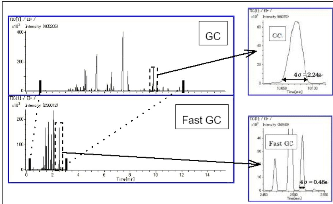
**Figure 1. GC and Fast GC: Analytical results and chromatogram peaks of B-Farnesene**
