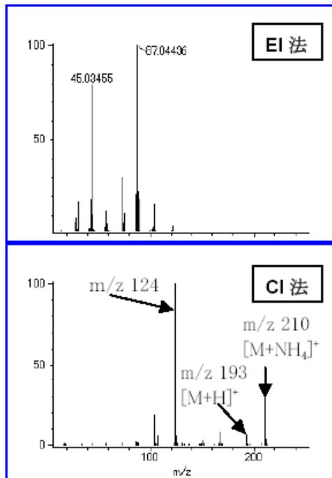
Figure 2. Mass spectra of unknown component in triethylene glycol
