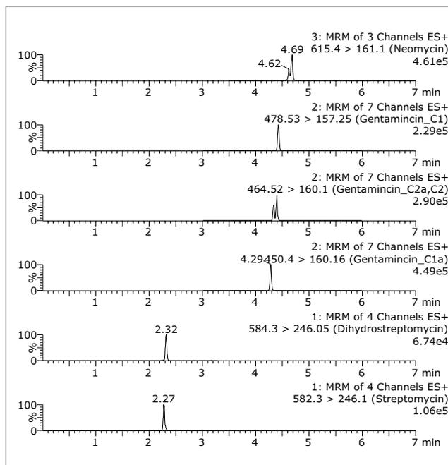
UPLC/MS/MS chromatogram obtained from bovine milk spiked at 10 µg/kg (ppb).
