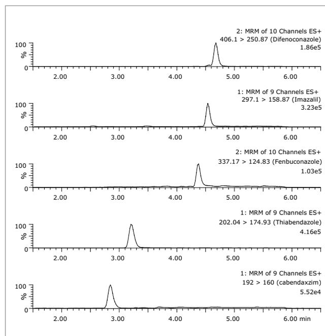
UPLC/MS/MS chromatogram obtained from DisQuE Pouch extract of orange juice spiked at 10 ng/g (ppb) of each fungicide (except 1 ppb carbendazim).
