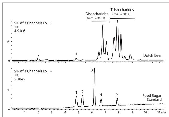
Figure 4. UPLC/MS analysis of carbohydrates in beer. Mobile phases are identical to Figure 3. Gradient from 10 to 70 % B in 10 minutes, reset and equilibrate for 25 minutes. The flow rate is 0.13 mL/min, the column temperature is 35 °C, and the Injection volume is 2 µL. The concentration of each analyte in the standard is 10 µg/mL in 50/50 ACN/H<sub>2</sub>O. The column dimensions are 2.1 x 100 mm, 1.7 µm. Peaks: (1) fructose, (2) glucose, (3) sucrose, (4) maltose, and (5) maltotriose.
