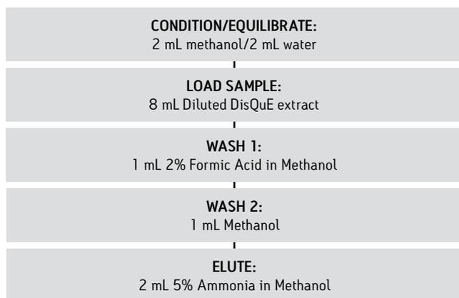
Figure 3. Oasis MCX SPE protocol for this study using a 3-cc cartridge.
