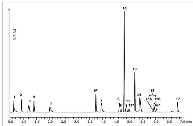
Chromatogram showing solvent standards with concentrations of approximately 5 ng/µL. All extracted at 270 nm, except compounds 6, 12, and 16. \* Extracted at 205 nm. Extracted at 630 nm.
