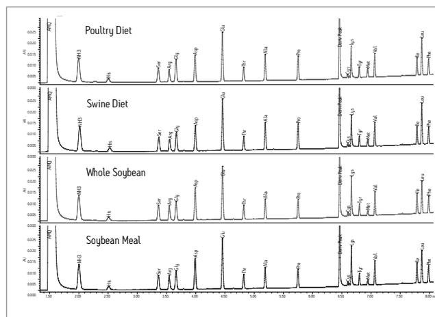
*Animal feed hydrolysates, 6 ng on column, using the UPLC Amino Acid Analysis Solution.*
