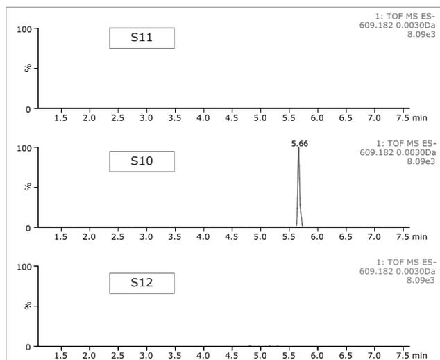
Extracted ion chromatograms (XIC) for  $m/z$  609.1816 (hesperidin) in S10, S11, and S12.
