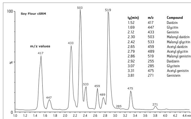
Figure 4. ESI-LC/MS confirmation of peak identity for the Soy Flour cSRM, using single ion recording (SIR).
