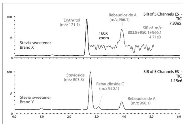
Figure 6. UPLC/MS analysis of two commercially-available stevia-related sweeteners. Isocratic mobile phase of 77.5/22.5 ACN/H<sub>2</sub>O with 0.1% NH<sub>4</sub>OH. The flow rate is 0.2 mL/min, the column temperature is 35 °C, and the Injection volume is 1.3 µL. The concentration of the Brand Y product is 50 µg/mL each in 50/50 ACN/H<sub>2</sub>O. The Brand X product is prepared at 10 µg/mL in 50/50 ACN/H<sub>2</sub>O. The column dimensions are 2.1 x 100 mm, 1.7 µm.
