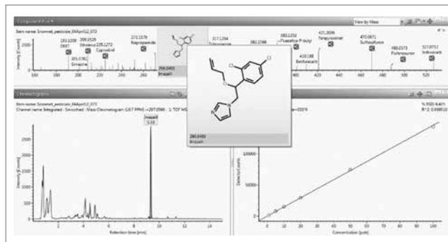
UNIFI component plot (upper data panel) shows the pesticide residues identified in a test sample and the calibration series for imazalil (1 to 100 ppb) and correlation coefficient  $R^2=0.999$ .
