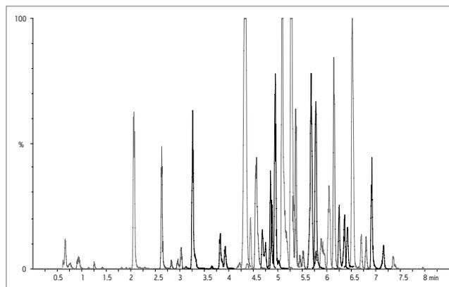
402 pesticide residues in one 10 minute run in injection solvent.
