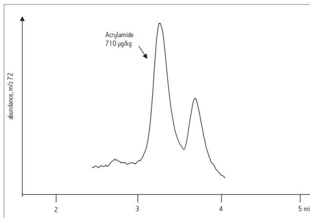
LC/MS determination of acrylamide in potato chips.
