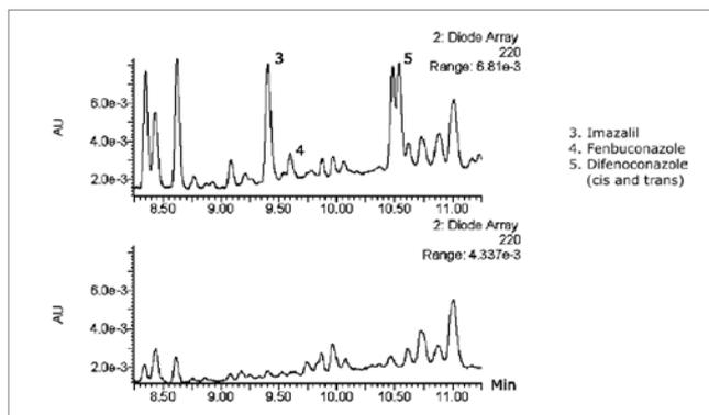
LC/UV (220 nm) chromatograms obtained on an *XP* Column from a *DisQuE* Pouch extract of orange juice spiked at 100 ng/g (ppb) after *Oasis* MCX cleanup.
