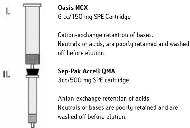
Tandem SPE Cartridges setup.
