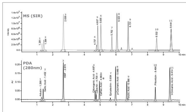
Simultaneous acquisition of PDA and MS (SIR) data for a 10 ppm standard mix in a single analysis.
