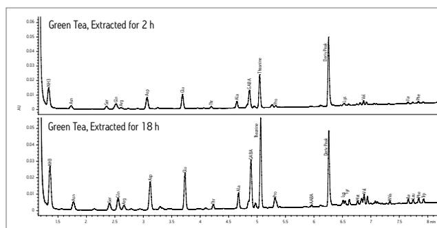
Two separate aliquots of a single type of green tea using the UPLC Amino Acid Analysis Solution. Each aliquot was extracted for 2 or 18 hours. Theanine (5.1 minutes) was confirmed by MS detection. All amino acid levels increase with duration of extraction.
