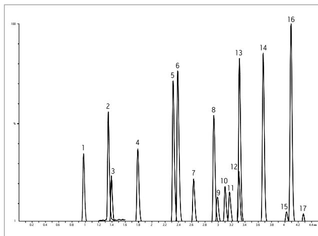
*17 pesticide residues in one injection at 1 ng/mL in water.*
