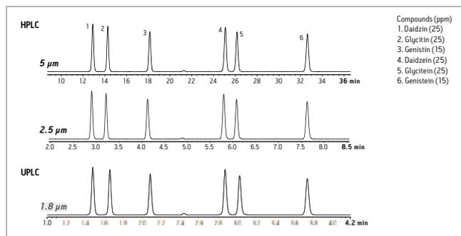
Figure 2. HPLC and UPLC separations (UV) of soy isoflavone standards on cyano columns: XSelect® HSS Cyano, 5 µm, 4.6 x 150 mm (top); XSelect HSS Cyano XP, 2.5 µm, 4.6 x 75 mm (middle); and ACQUITY UPLC HSS Cyano, 1.8 µm, 2.1 x 50 mm (bottom). The gradient profiles, flow rates, and injection volumes were scaled for each method using the ACQUITY UPLC Columns Calculator. The flow rates were 1.0 mL/min, 2.0 mL/min, and 0.58 mL/min, respectively.
