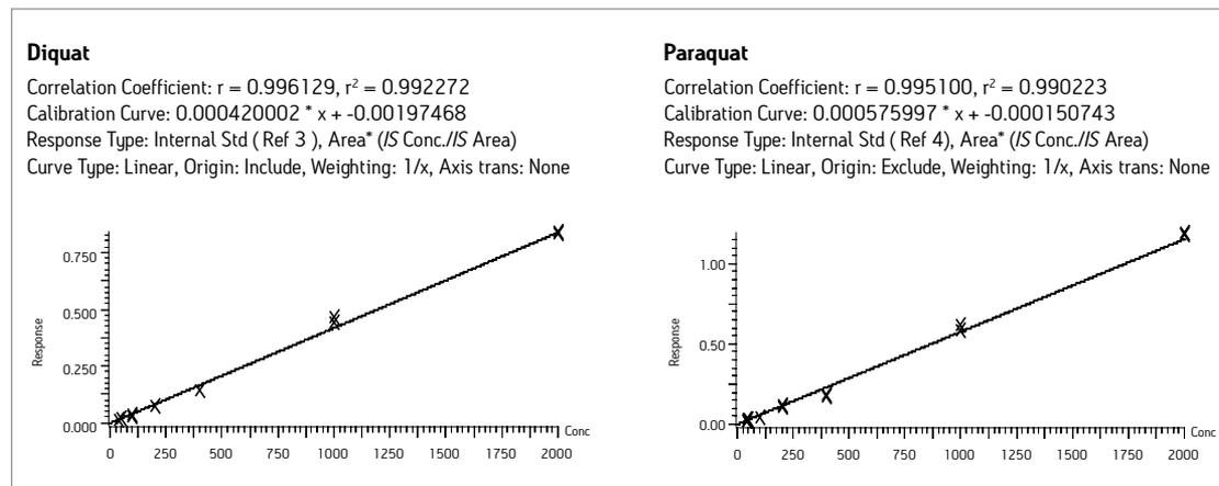
Figure 4. Typical LC/MS/MS Calibration Curves.
