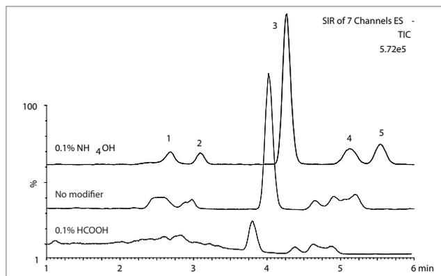
Figure 1. UPLC/MS analysis of carbohydrates in 75/25 ACN/H<sub>2</sub>O containing formic acid, no modifier, and ammonium hydroxide. The flow rate is 0.13 mL/min, the column temperature is 35 °C, and the Injection volume is 0.7 µL. The concentration of each analyte is 10 µg/mL in 50/50 ACN/H<sub>2</sub>O. The column dimensions are 2.1 x 50 mm, 1.7 µm. Peaks: (1) fructose, (2) glucose, (3) sucrose, (4) maltose, and (5) lactose.
