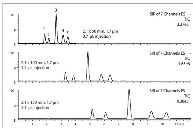
Figure 2. UPLC/MS analysis of carbohydrates using acetone as the organic solvent. The isocratic mobile phase was 77/23 acetone/H<sub>2</sub>O with 0.05% NH<sub>4</sub>OH. The flow rate is 0.13 mL/min and the column temperature is 85 °C. The column dimensions and Injection volumes are shown on the figure. The sample and peak elution order is identical to Figure 1.
