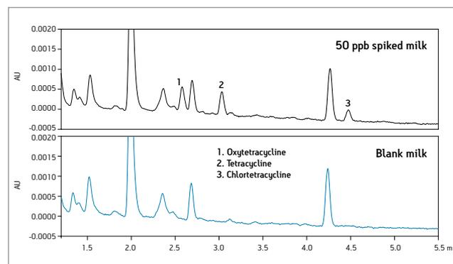
A typical HPLC/UV chromatogram (355 nm extracted wavelength, *XP* Column) obtained from analysis of a sample spiked with 50 ppb (ng/g) of three tetracyclines.
