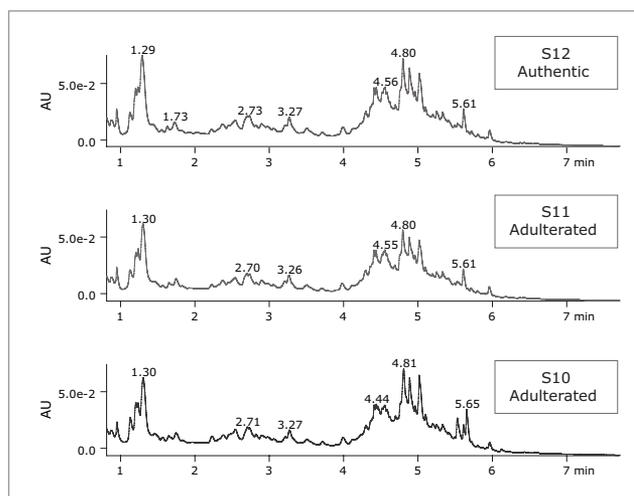
UV comparison (extracted wavelength – 283 nm) of three pineapple juices: S10, S11, and S12 (authentic sample).
