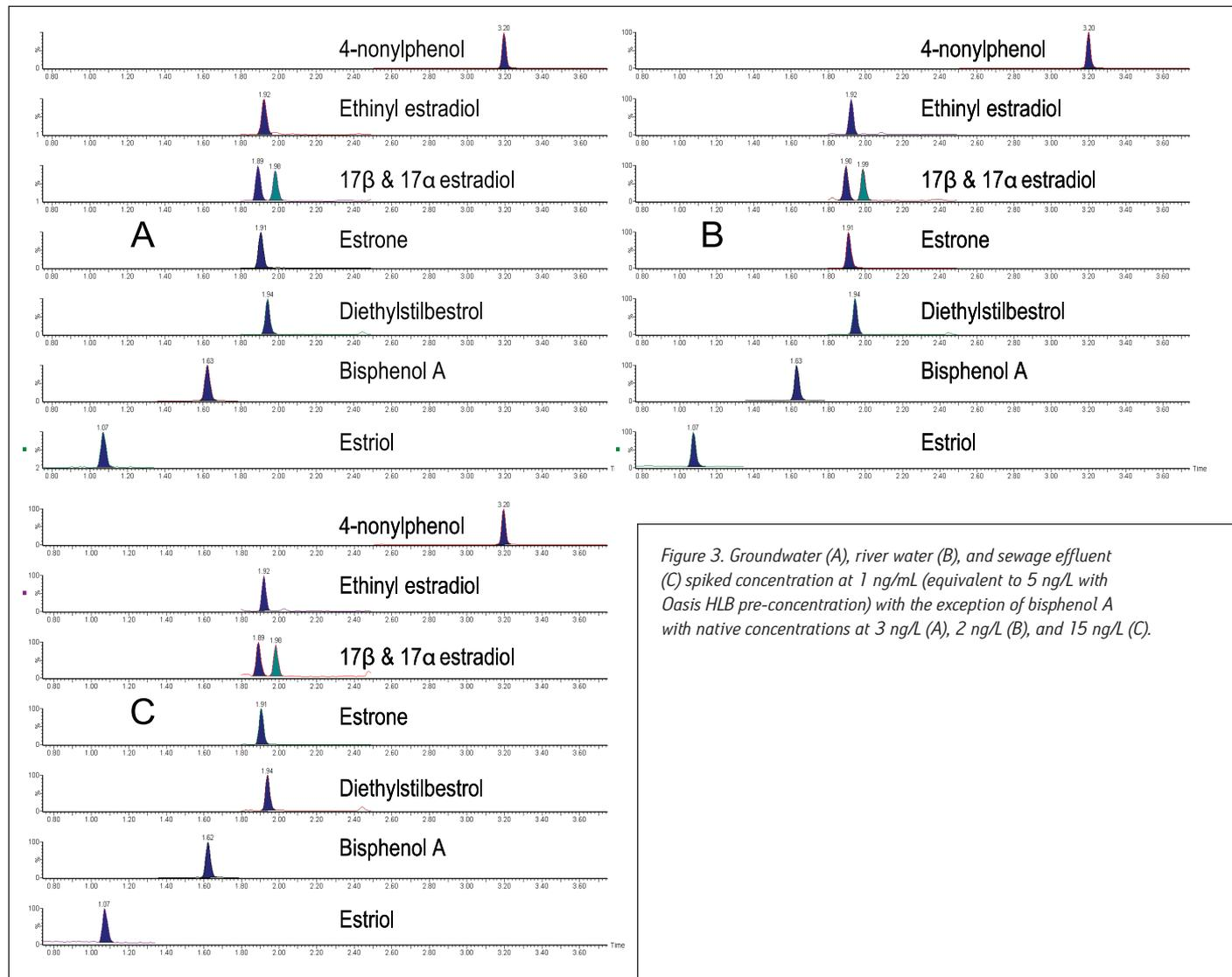
Figure 3. Groundwater (A), river water (B), and sewage effluent (C) spiked concentration at 1 ng/mL (equivalent to 5 ng/L with Oasis HLB pre-concentration) with the exception of bisphenol A with native concentrations at 3 ng/L (A), 2 ng/L (B), and 15 ng/L (C).
