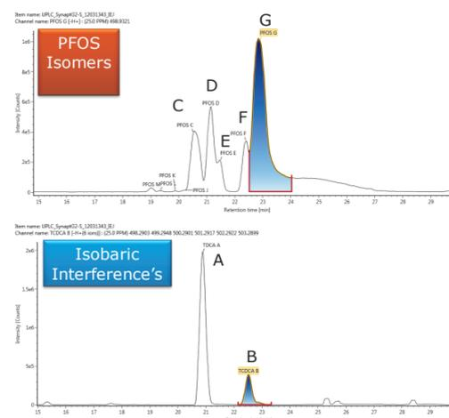
Figure 2. Accurate mass extracted ion chromatograms for the isobaric matrix interferences (Peaks A & B) and the PFOS isomers (Peaks C-G).
