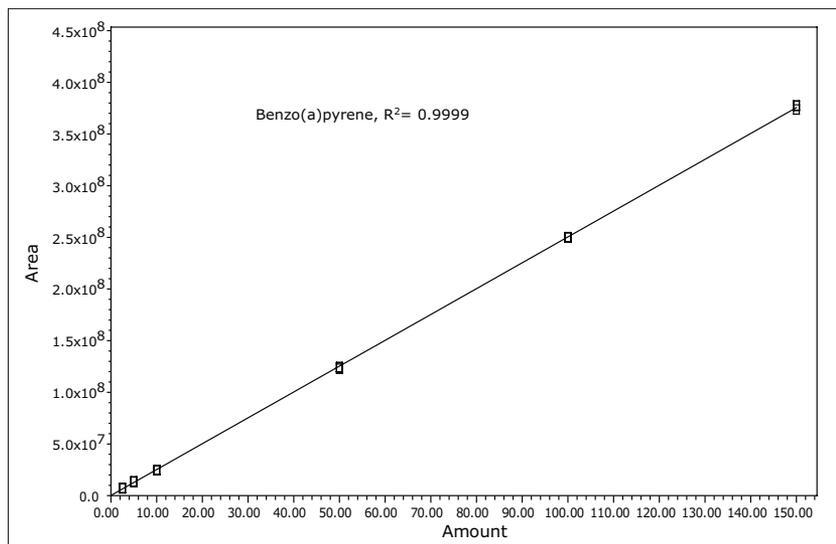
Figure 5. Calibration curve for benzo(a)pyrene (2.5 to 150.0  $\mu\text{g/L}$ ).
