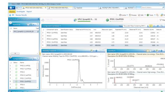
Figure 4. At 20.21 mins minor PFOS J (3mPFOS) isomer HDMS<sup>E</sup> fragmentation spectra that are ion mobility resolved from co-eluting PFOS isomer C.
