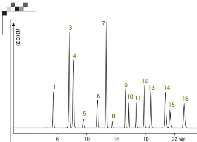
Standard chromatogram, fluorescence/programmed wavelengths, 1 to 20 ppm PAH analytes.
