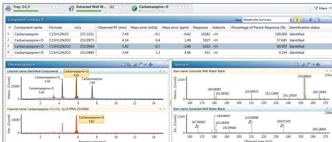
Figure 4. Full user interface (UI) information within UNIFI showing identification details of a proposed carbamazepine metabolite. Component summary shows identification details while the chromatogram shows extracted ion chromatograms of all identified components with the component highlighted in the component summary. The spectra section shows precursor and fragmentation spectra for the highlighted component.
