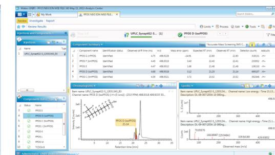
Figure 7. At 21.14 mins PFOS D (IsoPFOS) isomer HDMS<sup>E</sup> precursor ion and fragmentation spectra that are ion mobility resolved from co-eluting and isobaric TDCA.
