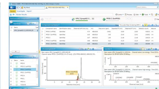
Figure 6. PFOS C (5mPFOS) isomer HDMS<sup>E</sup> precursor ion and fragmentation spectra that are ion mobility resolved from co-eluting PFOS isomer J at 20.21 mins.
