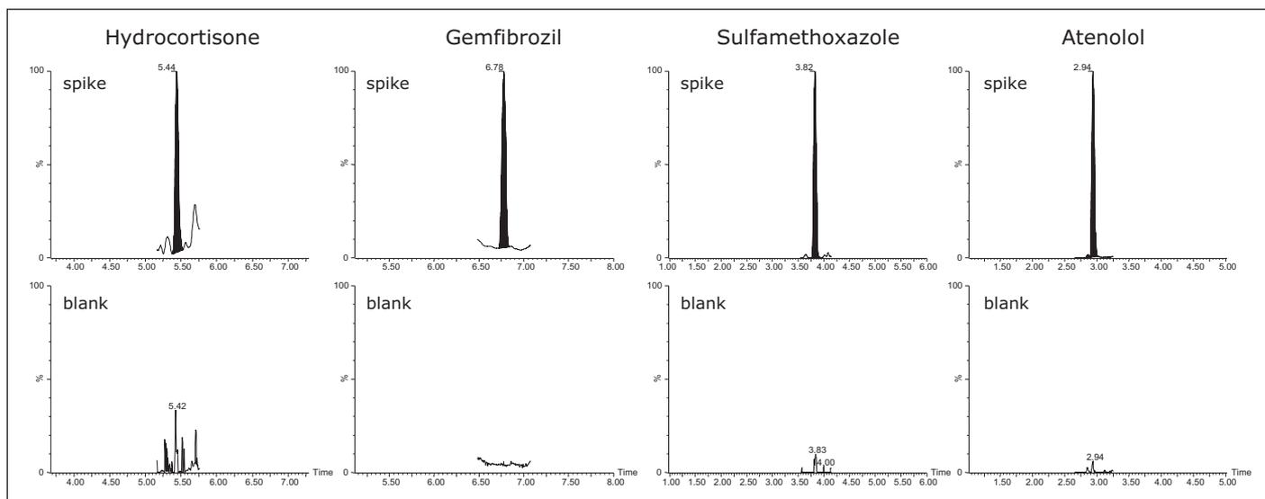
Figure 4. MRM chromatograms for example compounds that demonstrate blank responses in the extracted reagent water. The chromatograms in the top row demonstrate the expected response for the example compounds at the 0.1 ppt level (post-spiked into extracted reagent water). The bottom row shows the response in the blank extract of the reagent water.
