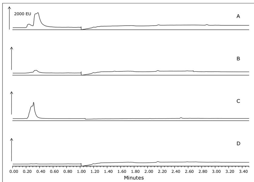
Figure 4. Chromatograms (A) unspiked shrimp, (B) fish, and (C) oysters carried through the QuEChERS procedure, along with a water blank (D). Changes in the baseline are a result of the programmed wavelength changes.
