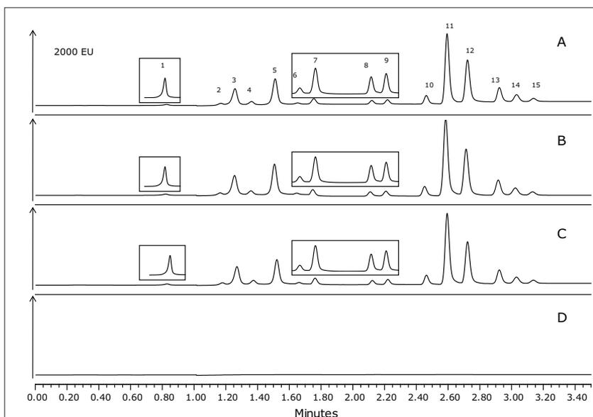
Figure 3. Chromatograms of PAHs spiked into (A) shrimp, (B) fish, and (C) oysters at 10.0  $\mu\text{g/g}$  (diluted 1:100 with acetonitrile following extraction). Insets show zoomed peaks for (1) naphthalene, (6) fluoranthene, (7) pyrene, (8) benzo(a)anthracene, and (9) chrysene. The blank water sample (D) taken through the extraction procedure is also shown.
