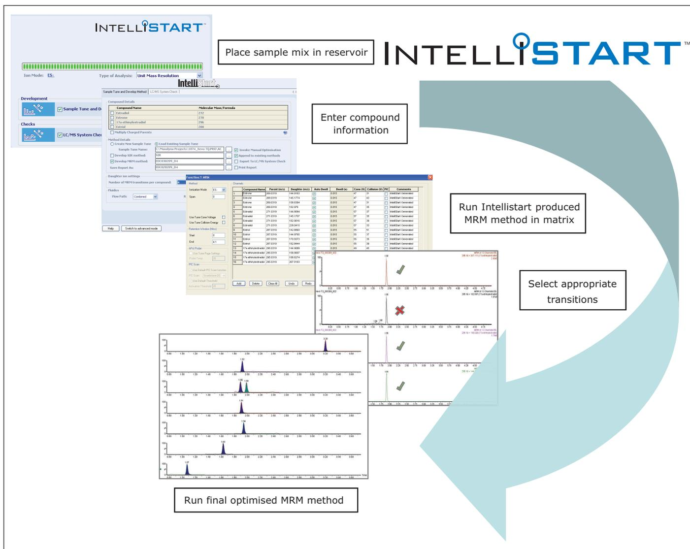
Figure 2. IntelliStart method development workflow on Xevo TQ MS.
