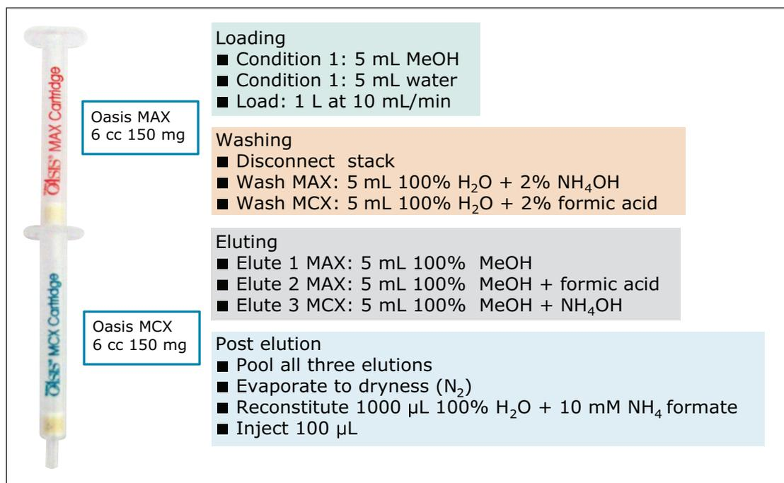
Figure 2. Schematic of solid phase extraction protocol for PPCPs in water.
