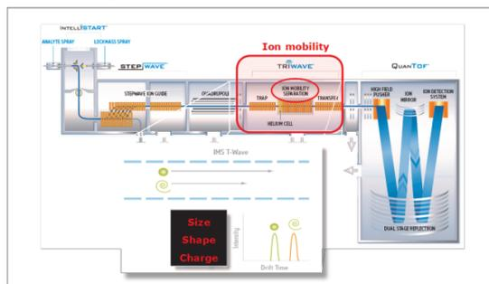
Figure 1. A schematic representation of the SYNAPT G2-S HDMS system and illustration of the mechanism of travelling wave ion mobility separations.
