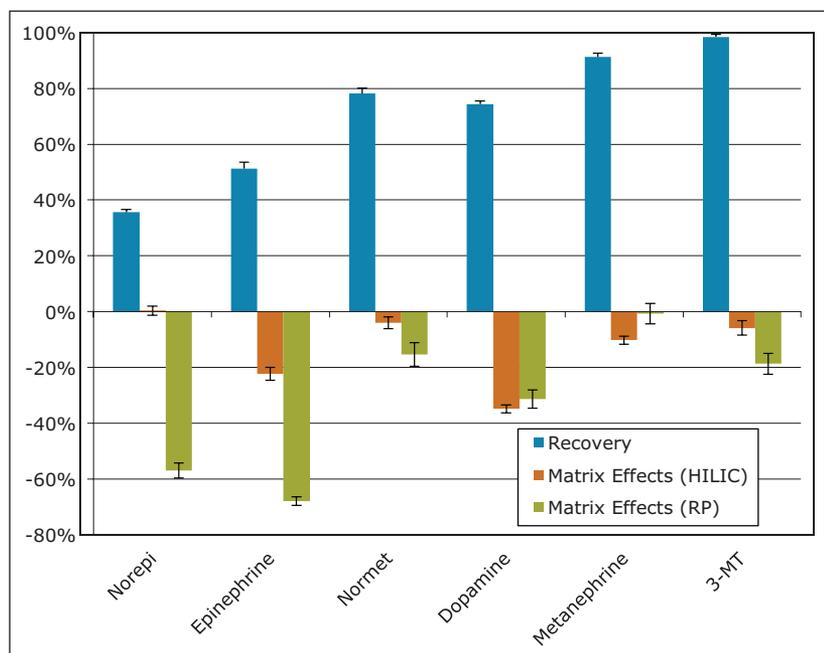
Figure 3. Recovery and matrix effects for catecholamines and metanephrines extracted from urine using Oasis WCX 30 mg 96-well Plates (N=4). The green bars represent matrix effects for reversed-phase analysis. Error bars indicate standard deviations.
