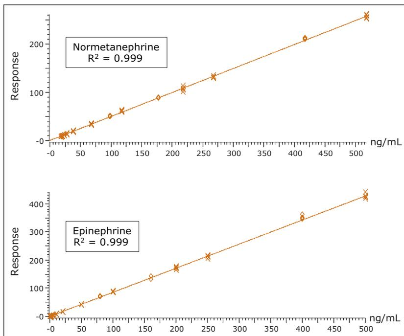
Figure 4. Calibration curves for normetanephrine (NMT) and epinephrine (EP) extracted from spiked urine samples. The data were fitted with a 1/x weighted linear fit. Basal concentrations for NMT and EP were 17.8 and 0 ng/mL, respectively.
