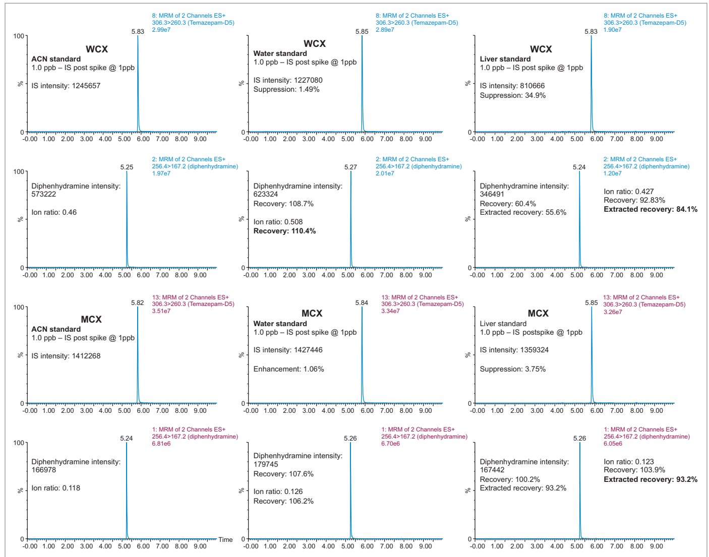
Figure 7. MCX vs WCX Chromatogram for MeOH std, water extracted std water, and matrix match extracted std for Diphenhydramine.
