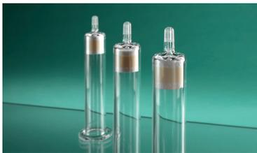
Fats and phospholipids are significant potential instrument and column contaminants. Oasis PRiME HLB Cartridges provide a rapid cleanup to remove these substances from meat extracts prior to LC-MS analysis.
