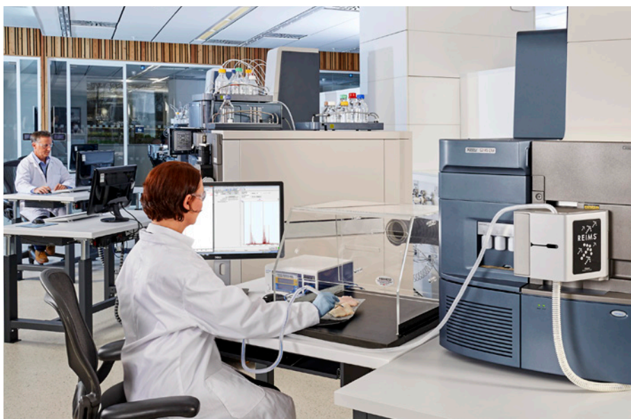
Rapid Evaporative Ionization Mass Spectrometry (REIMS) Research System with the hand-held iKnife.
