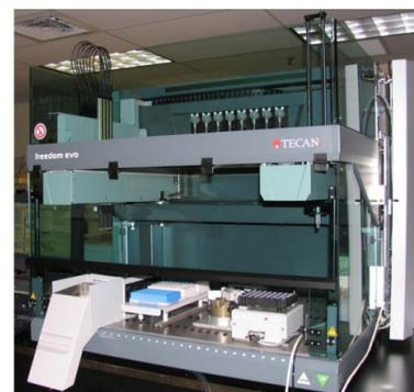
Figure 1. Tecan Freedom EVO system, as configured for amino acid analysis.
