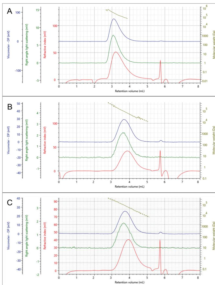
Figure 2. Overlaid chromatograms of the virgin polymer showing the UPLC (red) and analytical SEC (purple).
