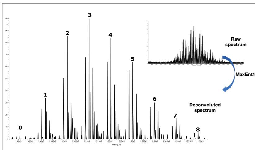
Figure 2. Raw and deconvoluted spectrum of LC(SEC)-MS analysis of Lysine conjugated ADC, Kadcyca (Trastuzumab Entansine (T-DM1)), by BioAccord System. The number labeled on the deconvoluted spectrum represents the detected number of drugs that are conjugated to the protein Trastuzumab in the intact level. The calculated average DAR is 3.46, vs. the published DAR of 3.50.<sup>3</sup> The experiment was conducted without deglycosylation of the ADC drug.
