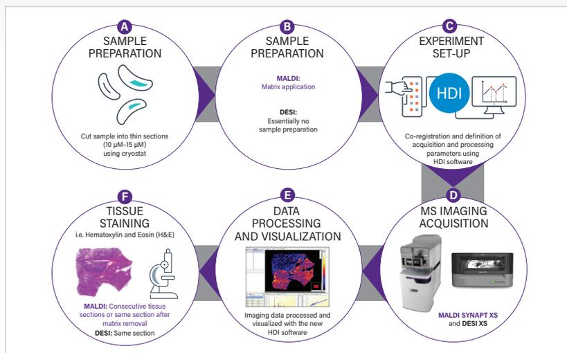
Figure 1. Full Spectrum Molecular Imaging workflow.
