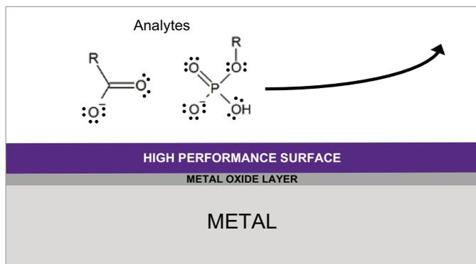
Figure 1. A MaxPeak High Performance Surface as utilized in the ACQUITY Premier Solution to impede electron rich analytes from interacting with metallic hardware.
