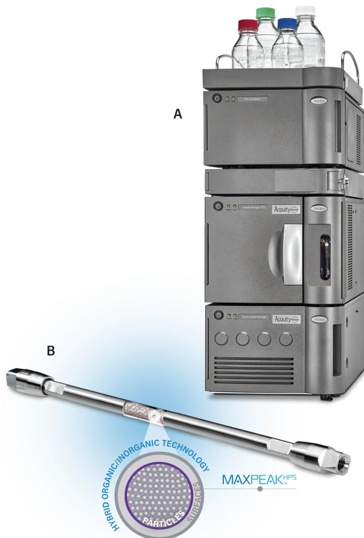
Figure 2. An ACQUITY Premier System and Column with MaxPeak HPS Technology. A) An LC instrument designed with a combination of corrosion-resistant components and hybrid organic/inorganic surfaces for sensitive, high efficiency RP and HILIC separations of metal-sensitive compounds. B) A complementary ACQUITY Premier Column constructed with hybrid organic/inorganic hardware surfaces.
